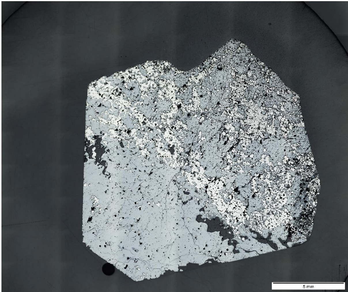
Figure 4.7: Blebby pyrite (pale yellow) throughout the massive sphalerite (dark grey), with gangue (black) of sample 395 in reflected light.
