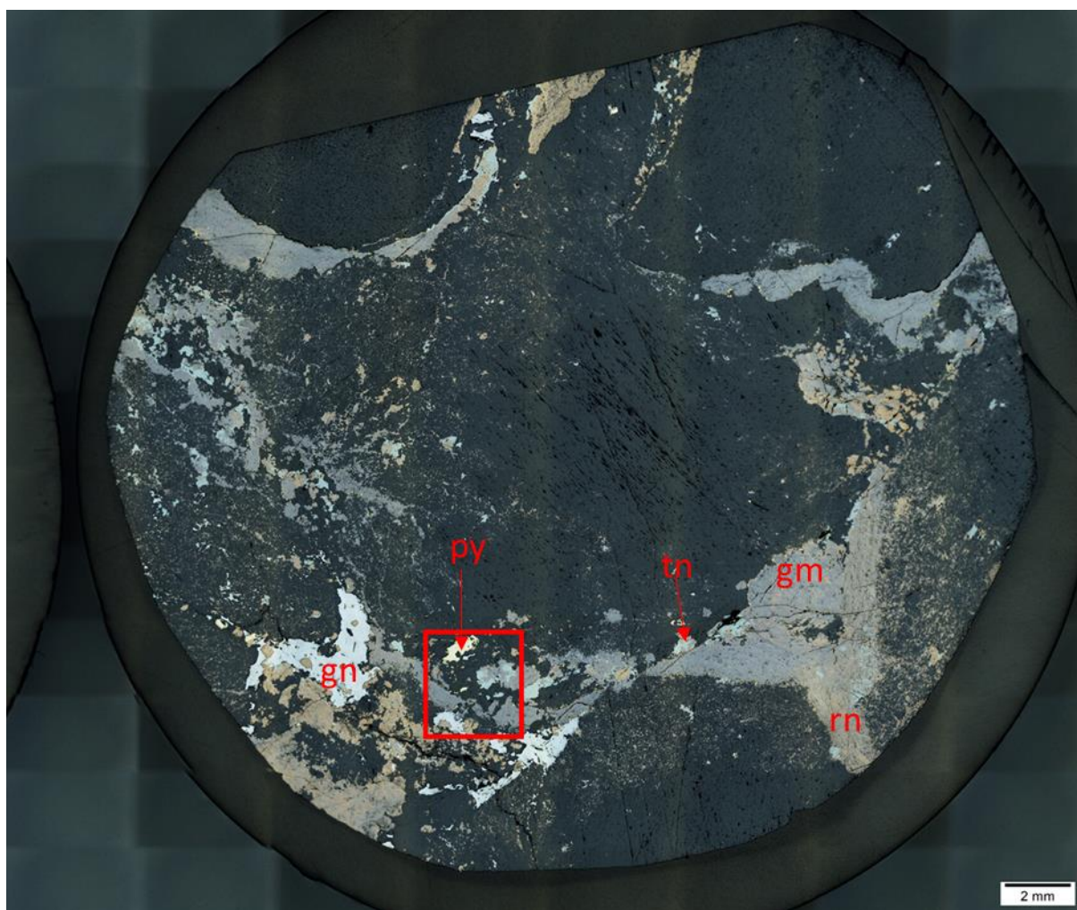
Figure 4.14: Full polished ore block reflected light image showing sample TS3 and the area selected for TIMA analysis (red rectangle).
