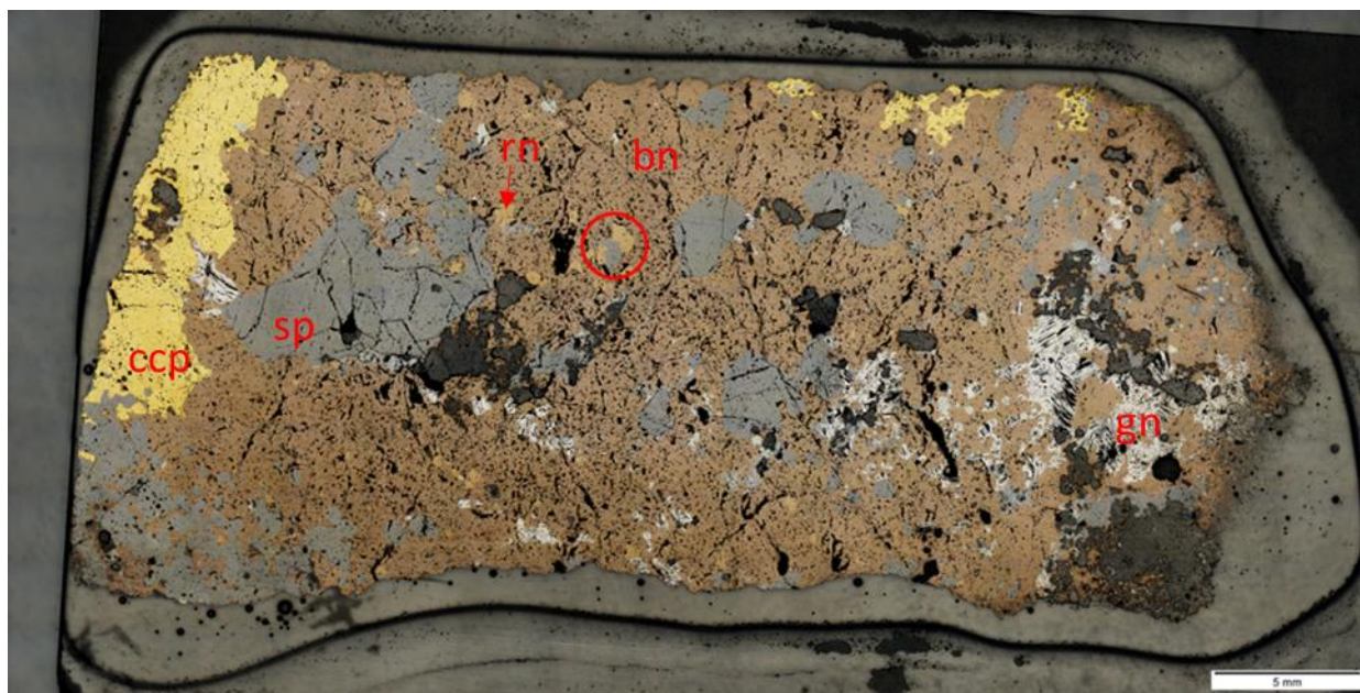
Figure 3.19 Full polished thin section image in reflected light showing bornite-dominant sample KP12 and the area selected for TIMA analysis (red circle).
