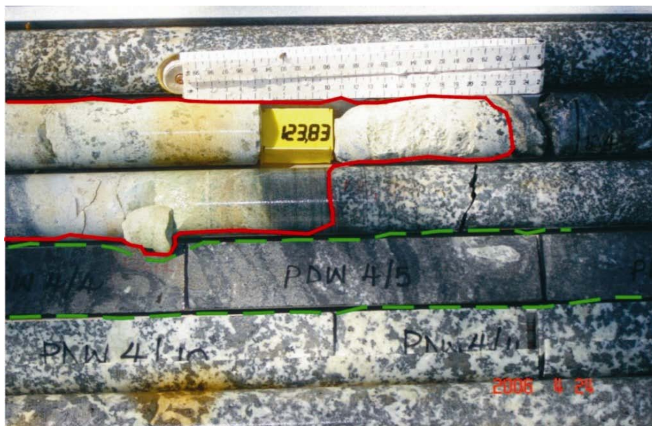
Figure 18: A calc-silicate xenolith that is rich in epidote (shown in red line) within a BC norite sequence in borehole PWD4. Part of the disturbed UG2 footwall with flow structures as defined by chromite and magnetite stringers is delineated by the dashed green lines.
