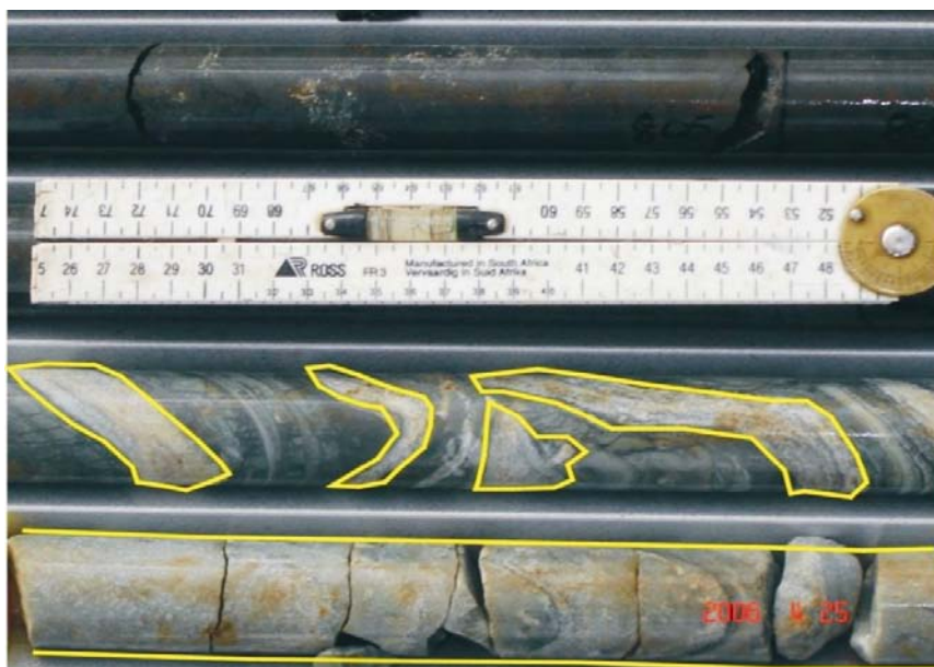
Figure 19: Diamond drill core of sedimentary xenoliths (in yellow) in core of the BC within Marginal Zone of the BC at De Wildt project. Below the xenoliths is part of the Transvaal Supergroup quartzite intersected in borehole DWD11.
