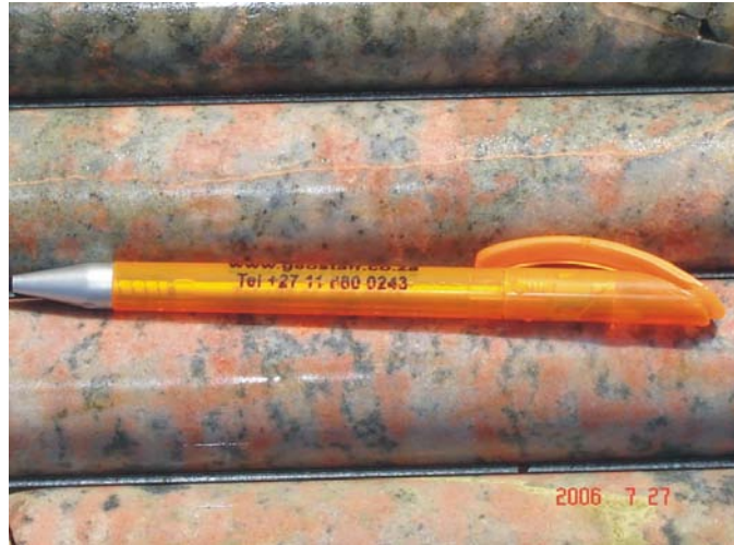
Figure 50: Potassic quartzite hornfels intersected in borehole at Krelingspost Farm. It is not known whether this unit is connected to the floor or comprises a Transvaal Supergroup outlier.
