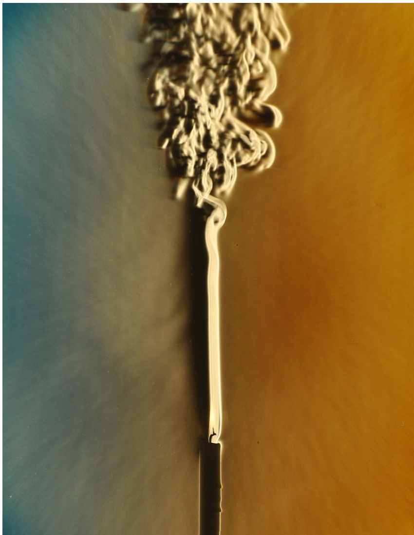
(B) "This Schlieren photograph shows the thermal convection plume rising from an ordinary candle in still air. The plume is initially laminar, but transition to turbulence occurs in the upper 1/3 of the image. The image was made using the 1-meter-diameter schlieren mirror of Floviz Inc. " by Dr. Gary Settles is licensed under CC BY-SA 3.0 .
