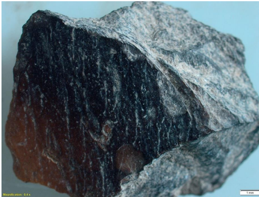
Figure A. 8: Displaying sheen as a result of burning.
