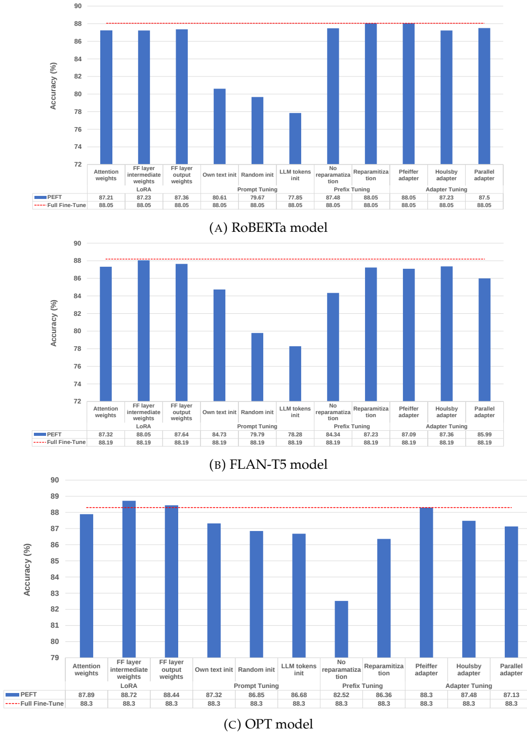
FIGURE 4.1: Modelling performance of PEFT methods and their various configurations with full fine-tuning as the baseline
