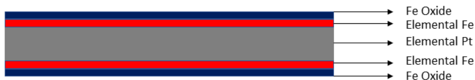
Figure 4.1: Schematic of the longitudinal cross-section of the prototype Fe coated Pt NWs depicting the layout of the core shell structure
