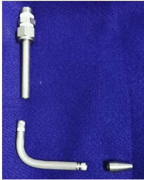
Figure 4-9 : Primary nozzle manufactured in three parts
