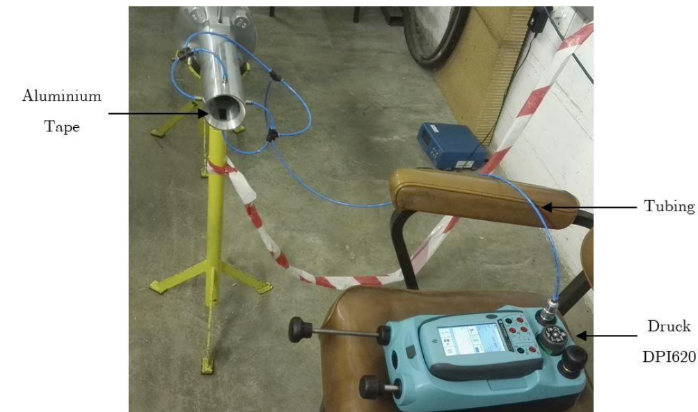
Figure 4-17 : Conical inlet tubing connection leak test setup
