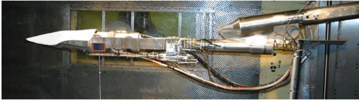
Figure 2-4 : Inlet test arrangement at the Calspan Transonic Wind Tunnel [4]
