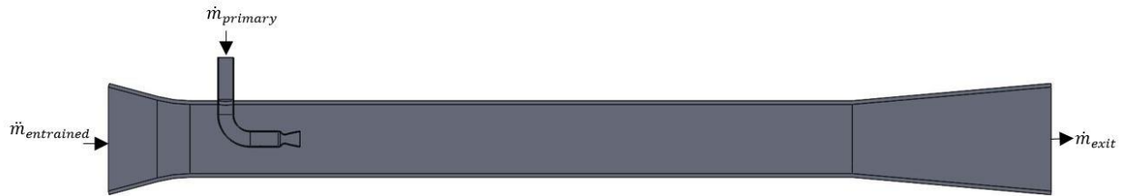
Figure 4-1 : Configuration of a single ejector with required mass flow rate determination points
