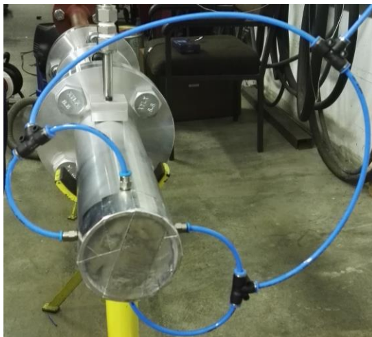
(a) Conical inlet entry sealed
