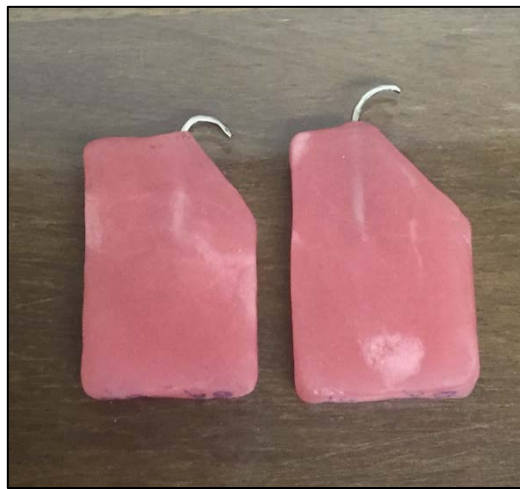
Figure 11. Permanent deformation of the premolar cast clasp on the right after it was displaced until its proportional limit was exceeded.
