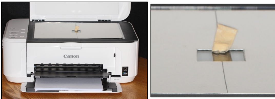
Figure 3. The dies being scanned on a flatbed scanner with the scanning template.
