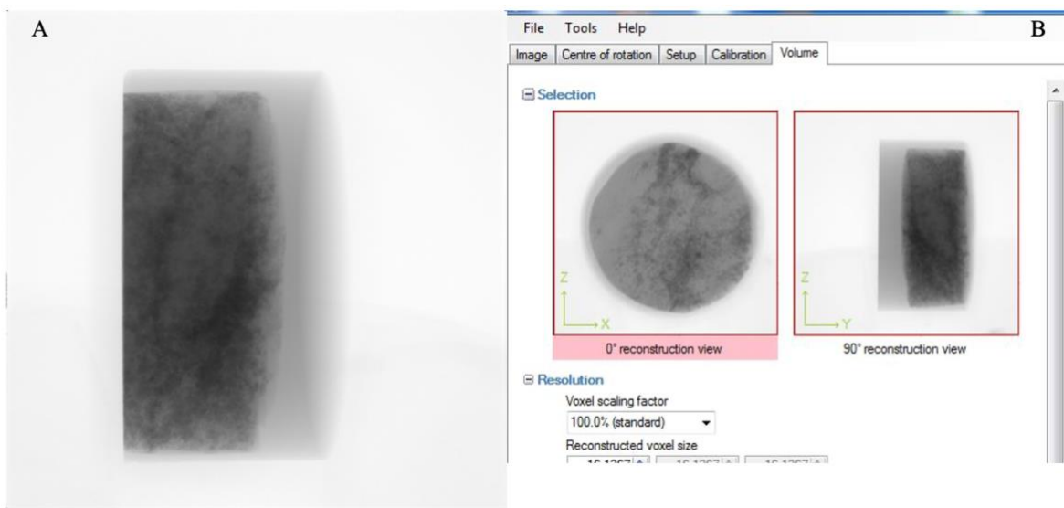
Figure 4.2: A) Raw CT data before conversion into slices. B) A screenshot of the image reconstruction process from the CT Pro 3D software.
