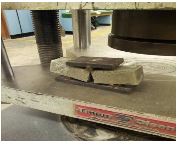
Figure 3.3.1—3: Splitting the Prism into Two Approximately Equal Portions (Two Twin Halves obtained)
