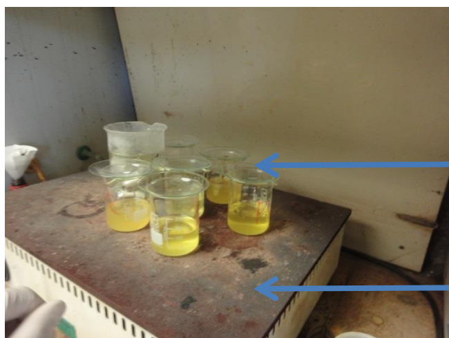
Figure 3.2.1—2: Illustration of Samples Allowed to be heated on Hot Plate
