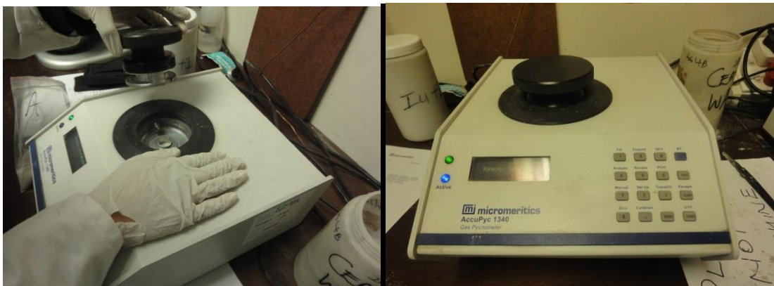
Figure 3.3.4—1: Illustration of the Gas Pycnometer used to infer the Density of the Cements
