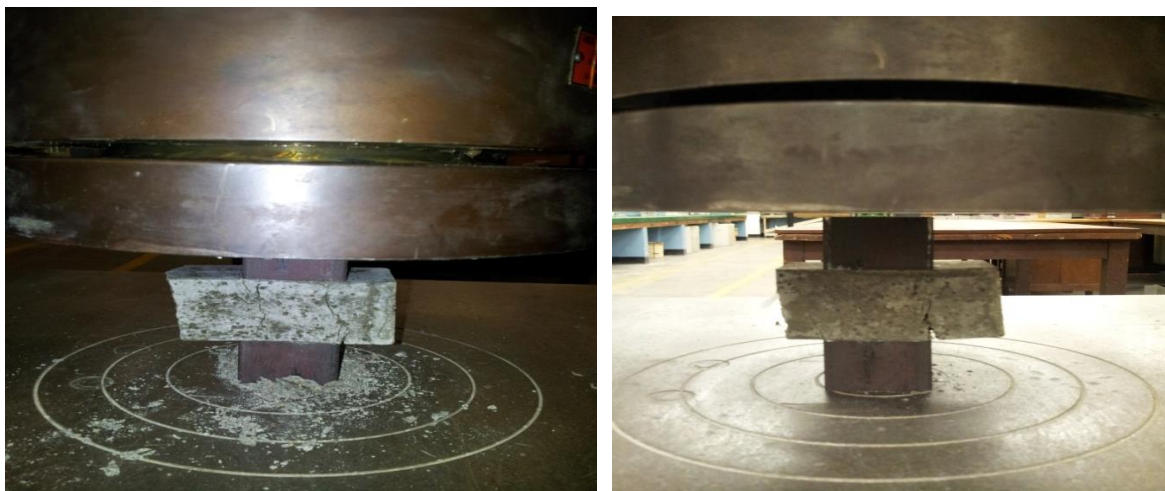
Figure 3.3.1—4: Twin Halves of Mortar cubes Under Compression
