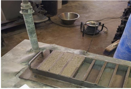
Figure 3.3.1—1: Specimen on Vibrating Table
