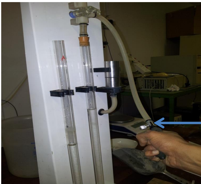
Figure 3.3.4—3: illustration of the Operator Using a Hand pump to Pass air into the Blaine Apparatus
