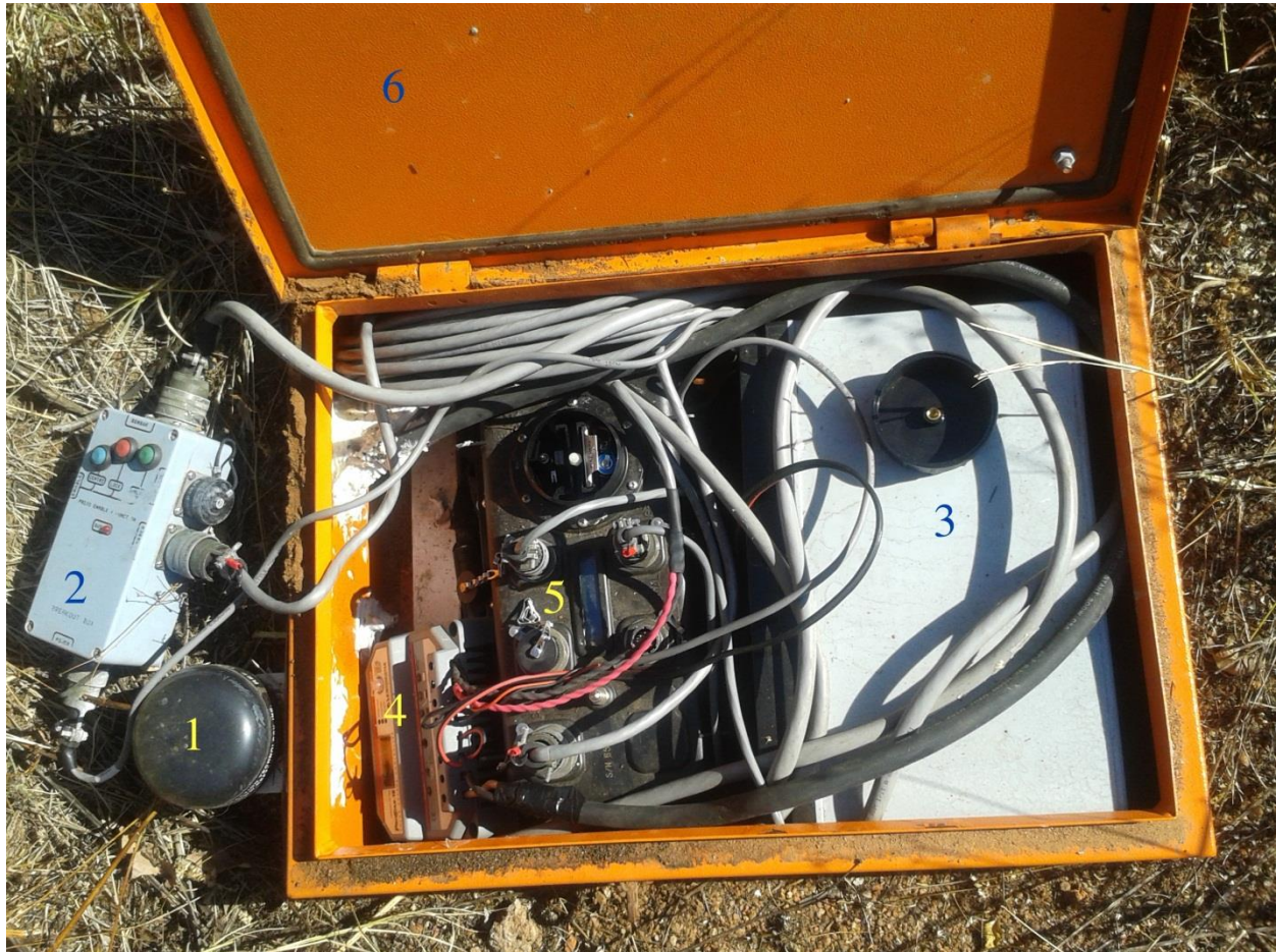
Picture 1. An example of complete seismic station deployed in sedimentary basin.
