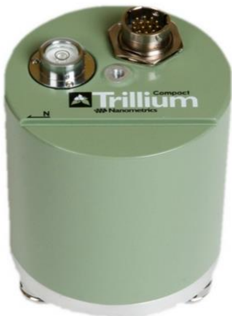
Picture 4. Broadband seismometer: Nanometrics Trillium Compact
