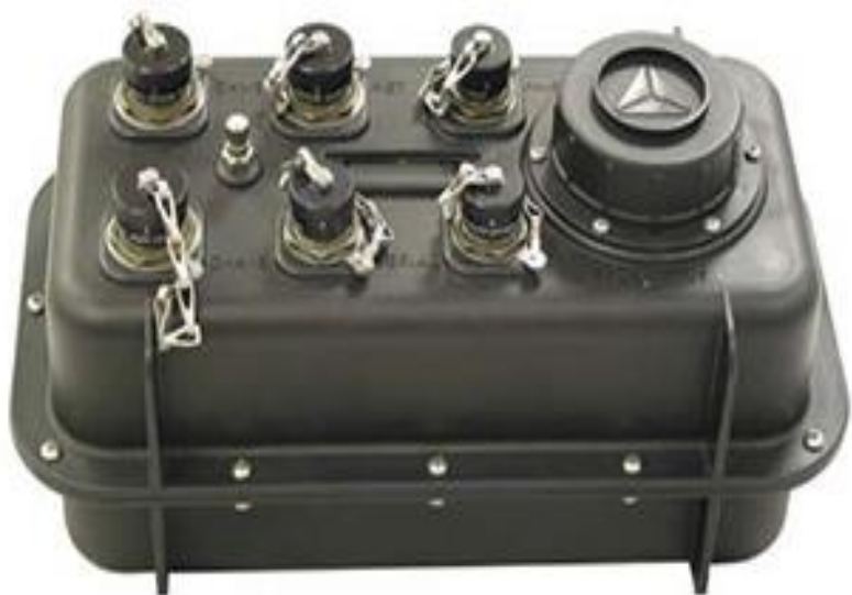
Picture 5. Data logger 24 – bit Reftek 130
