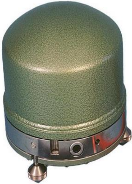
Picture 2. Broadband seismometer: Streckeisen STS – 2 G1.
