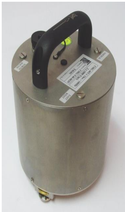
Picture 3. Broadband seismometer: Guralp CMG – 40T.
