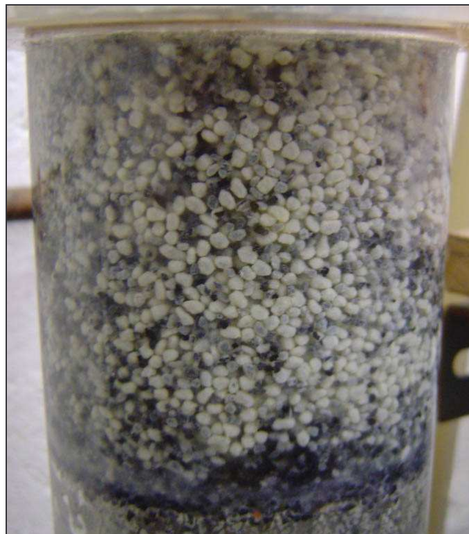
Figure 3.6: Biofilm development on GAC particles in the AFBR.
