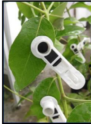
Figure 16. The clip of the fluorometer attached to the leaf of a eucalypt.
