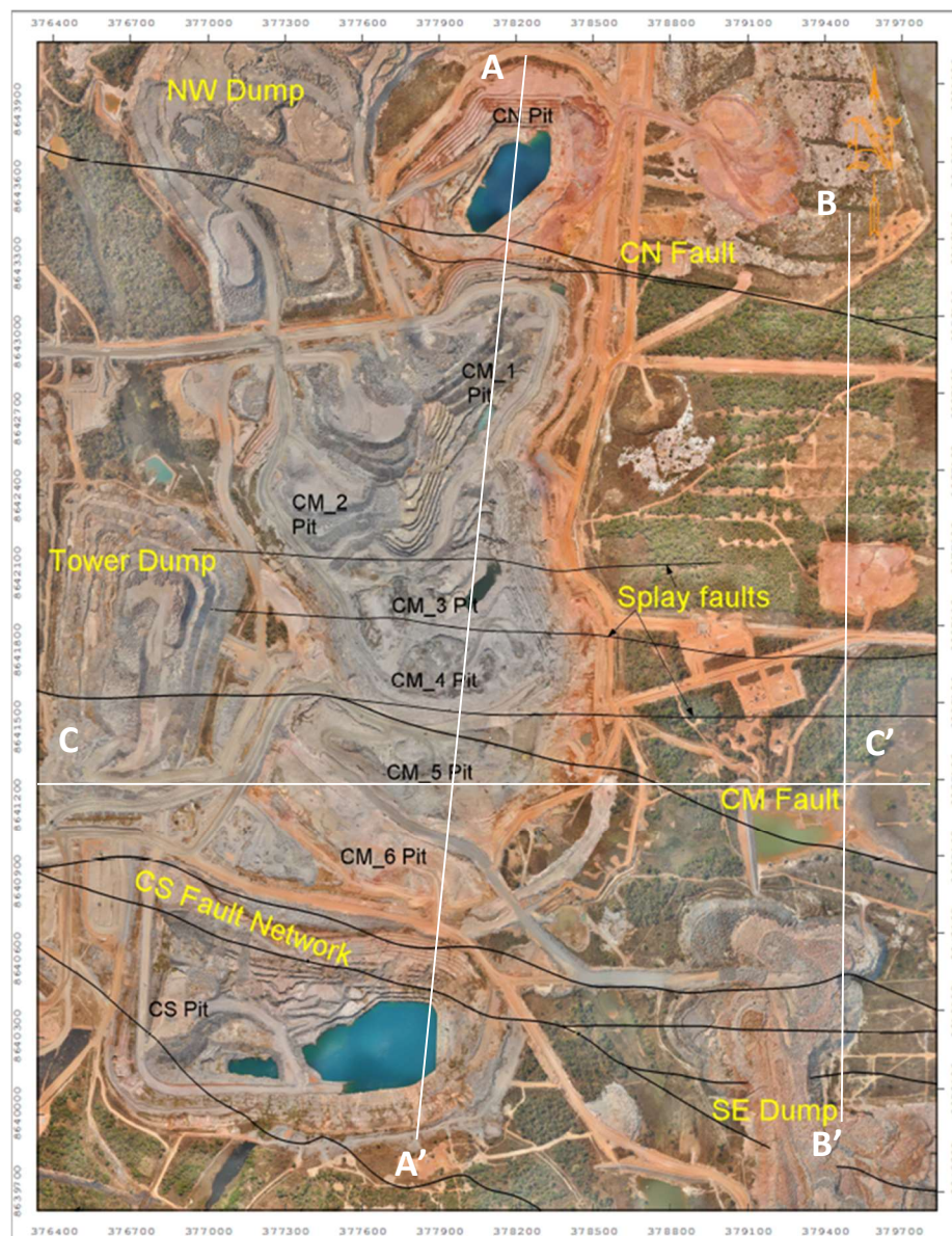
Figure 5.8. An aerial photo of the Chimiwungo pits overlaid by the major fault and some of the minor (splay) fault traces (Black lines). The aerial map is courtesy of the Lumwana Mining Company Survey team. CN = Chimiwungo North; CM = Chimiwungo Main; CS = Chimiwungo South. The section lines AA' and BB' are drawn through the high Cu concentration zones which flank the eastern aspect of both Shoots. The two section lines are shown in Figure 5.9a and b. Section line CC' defines a section across the deposit shown in figure 6.3.
