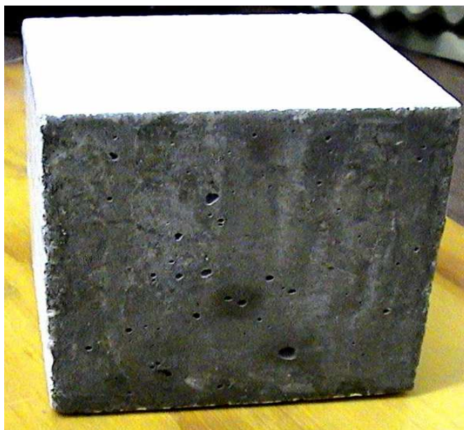
Figure 5.1 Concrete cube prepared for surface leaching for Cr(VI) content.
