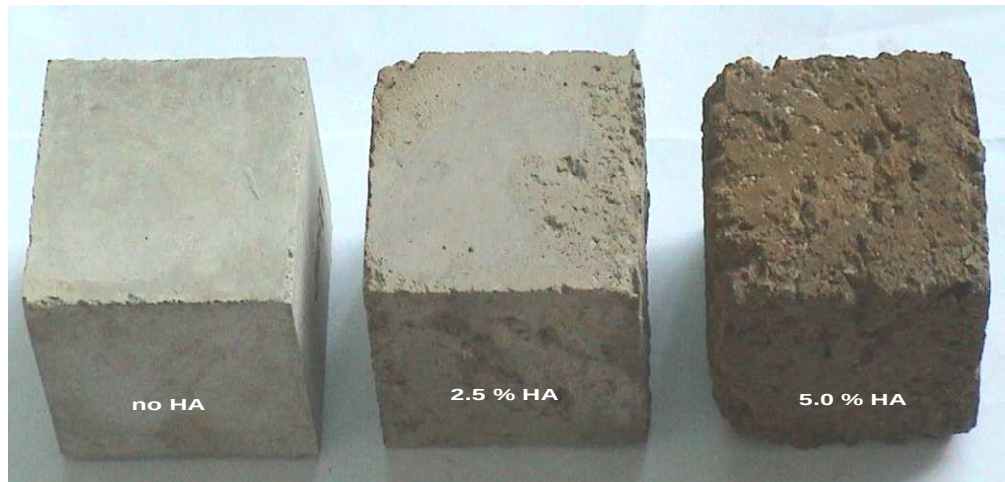
Figure 5.13 HSC01 concrete cubes consisting different amount of HA: no HA, 2.5 % HA and 5 % HA, respectively.
