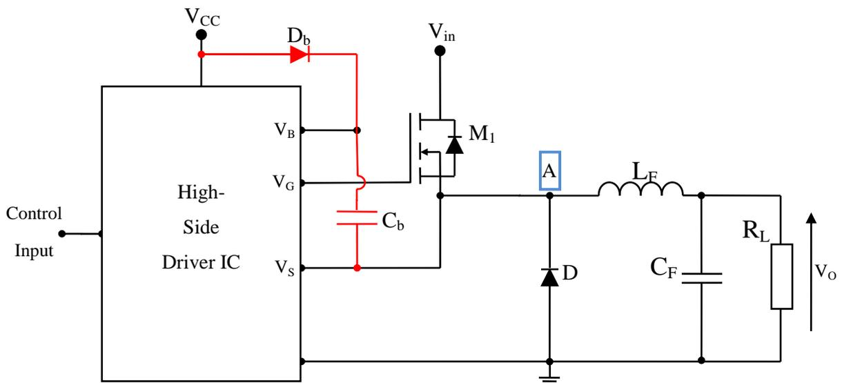
Figure 4.3: Typical high-side driver implementation
