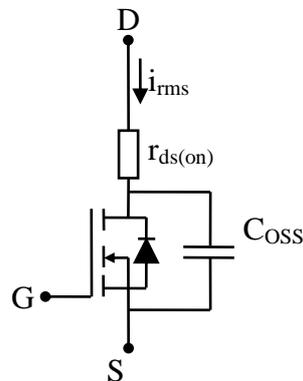
Figure 3.9: MOSFET model with losses
