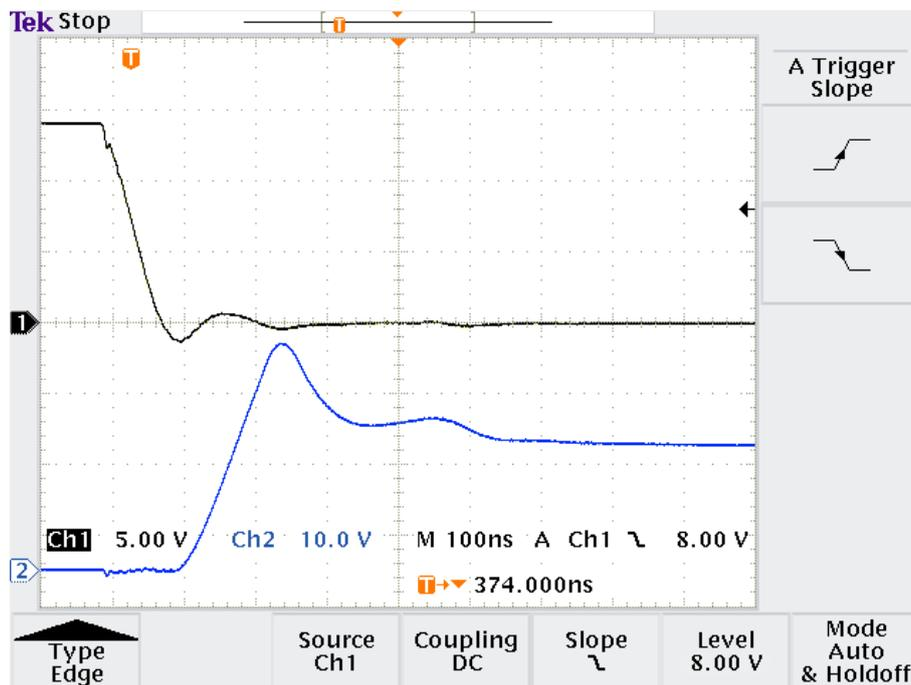
**Figure A.10: Gate and  $V_{DS}$  voltage for the low side MOSFET (Turn off transition)**
