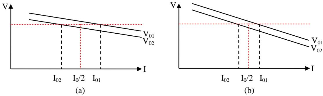
**Figure 4.18: The droop current sharing method (a) with a shallow voltage regulation curve. (b) with a steep voltage regulation curve [19].**
