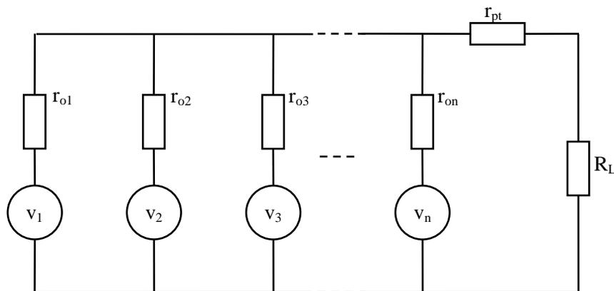
Figure 3.12: Origin and position of the power-train and output resistances in the multi-node converter model
