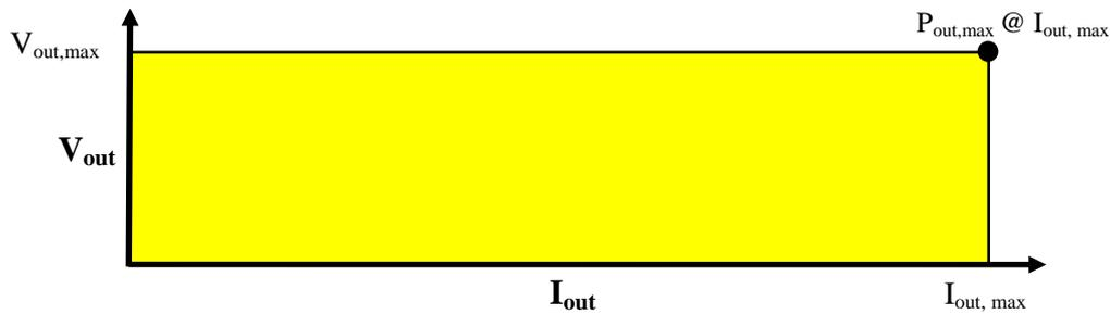
Figure 1.1: The V-I curve for a generic converter.
