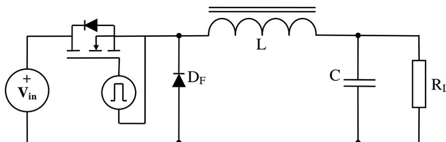
Figure 1.5: A standard Buck Converter
