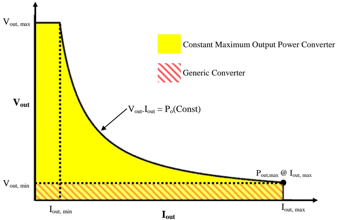
**Figure 1.3: A V-I curve for constant maximum output power**
