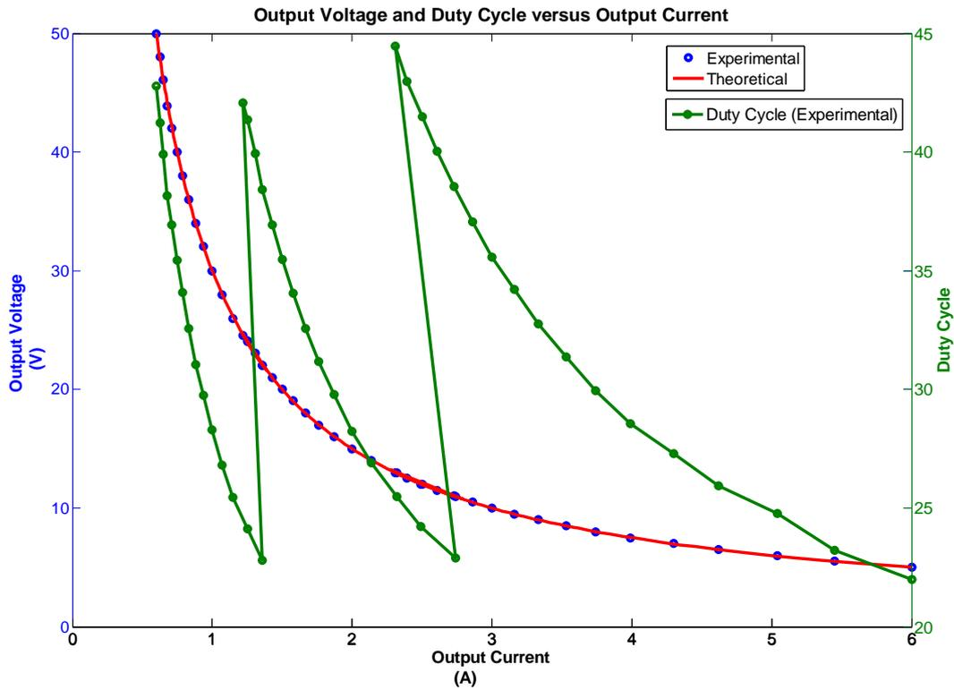
**Figure 5.3: Output voltage versus output current showing a constant power output**
