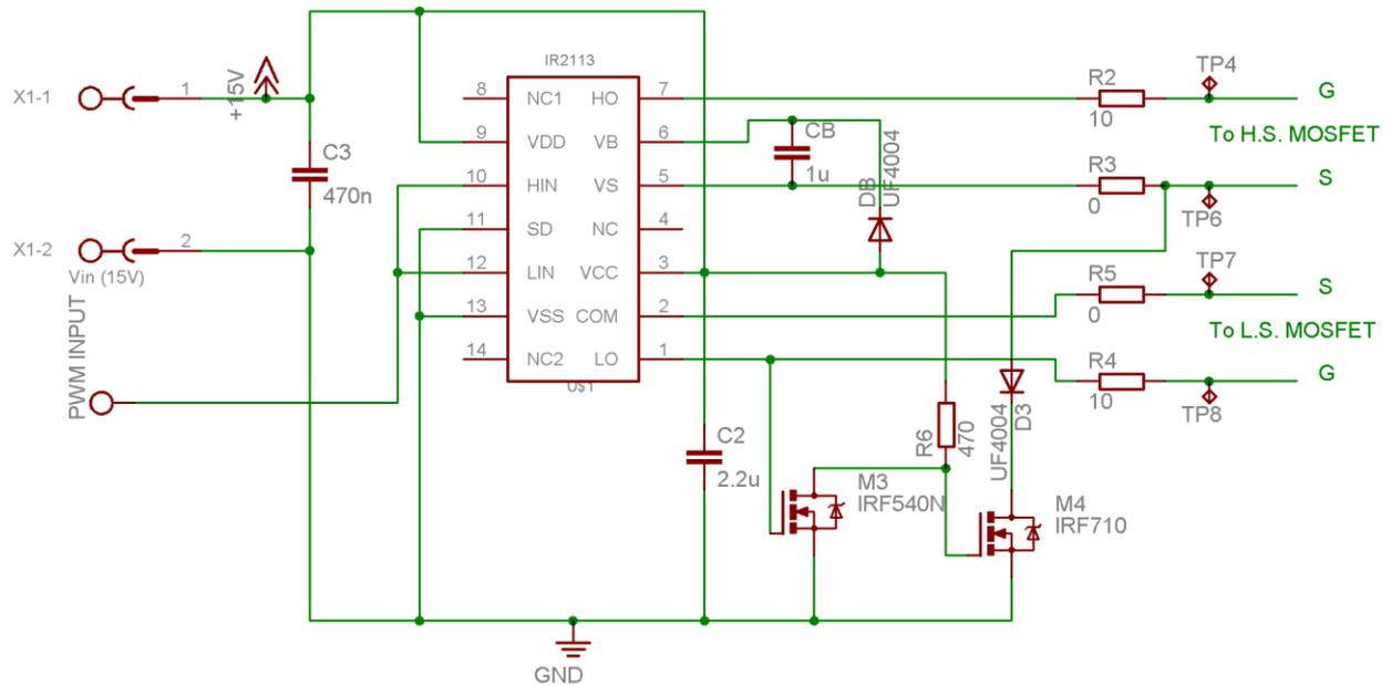
**Figure B.3: Driver schematic**
