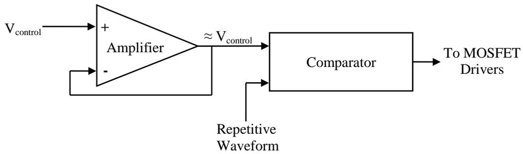
**Figure A.2:** A schematic showing open loop control of a SMPS
