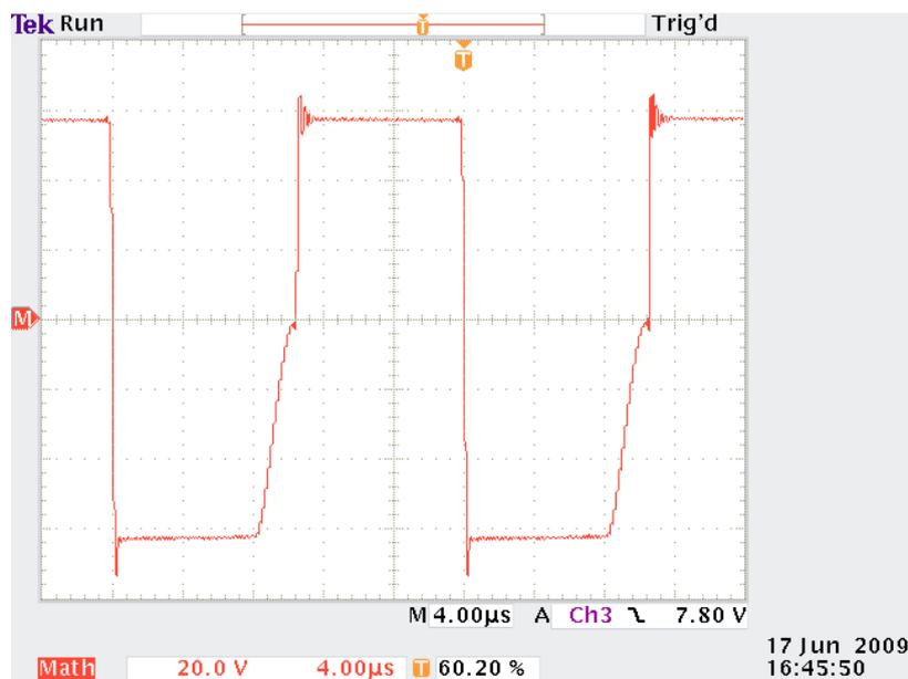
**Figure 4.15: Transformer output voltage with the series diode modification**
