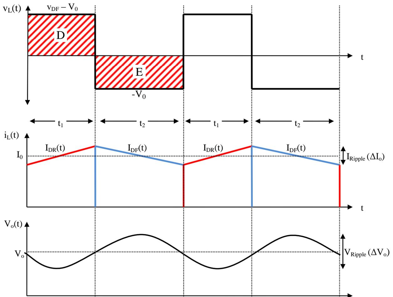
Figure 3.6: Filter waveforms in the Continuous Conduction Mode (CCM)
