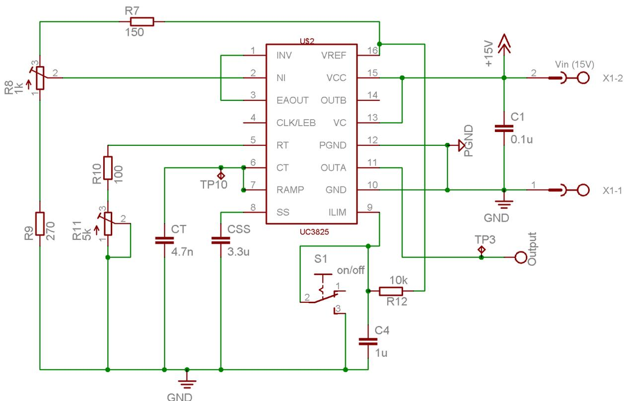
**Figure B.2: Controller schematic**
