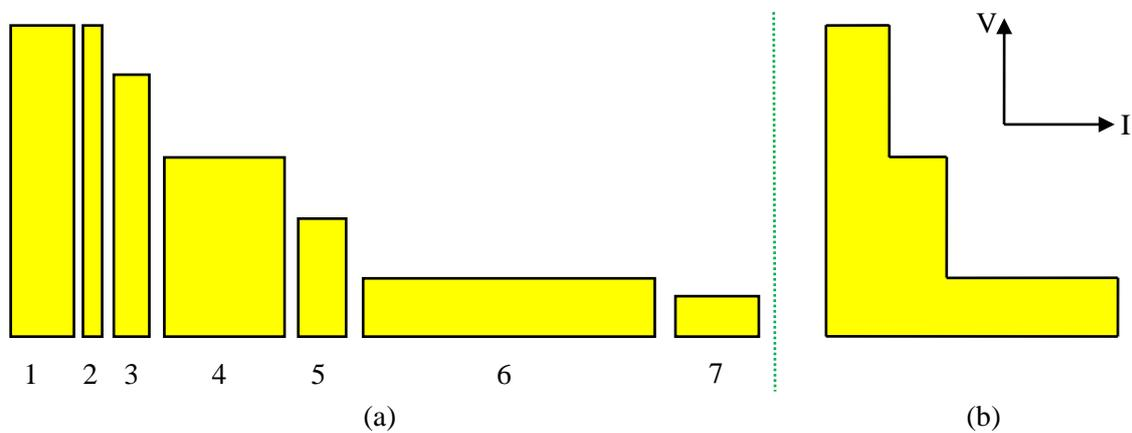
Figure 2.10: (a) Possible V-I curves for all of the different switch positions. (b) The final V-I curve.
