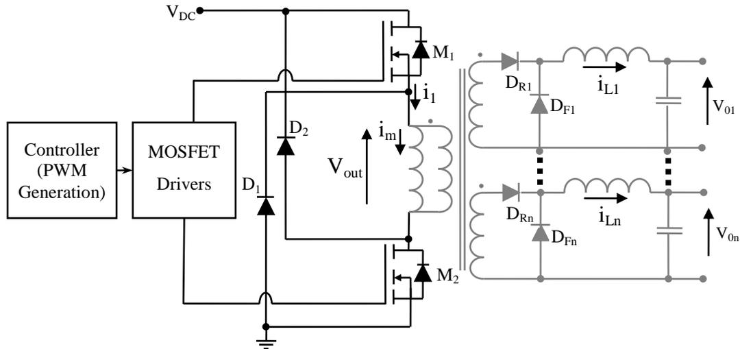
Figure 4.2: The two-switch forward converter test platform
