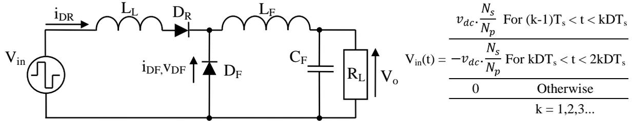
**Figure 3.3: A single phase forward converter model with the transformer’s leakage inductance included**
