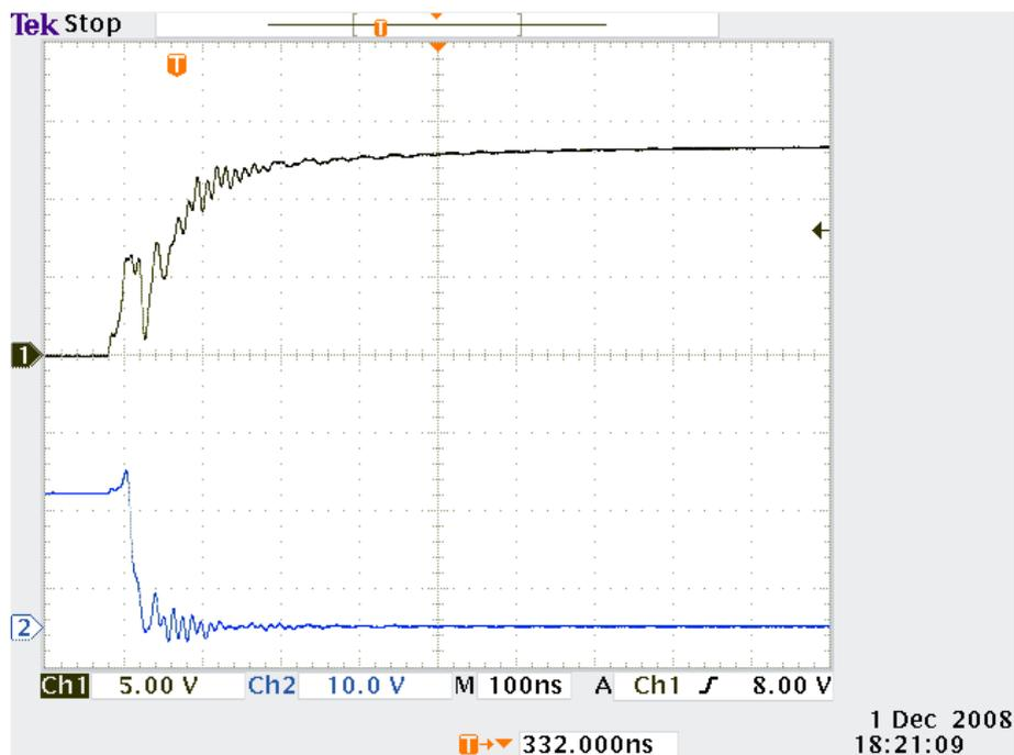
Figure A.9: Gate and  $V_{DS}$  voltage for the low side MOSFET (Turn on transition)
