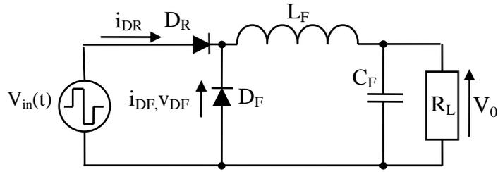
Figure 3.5: Single phase forward converter model
