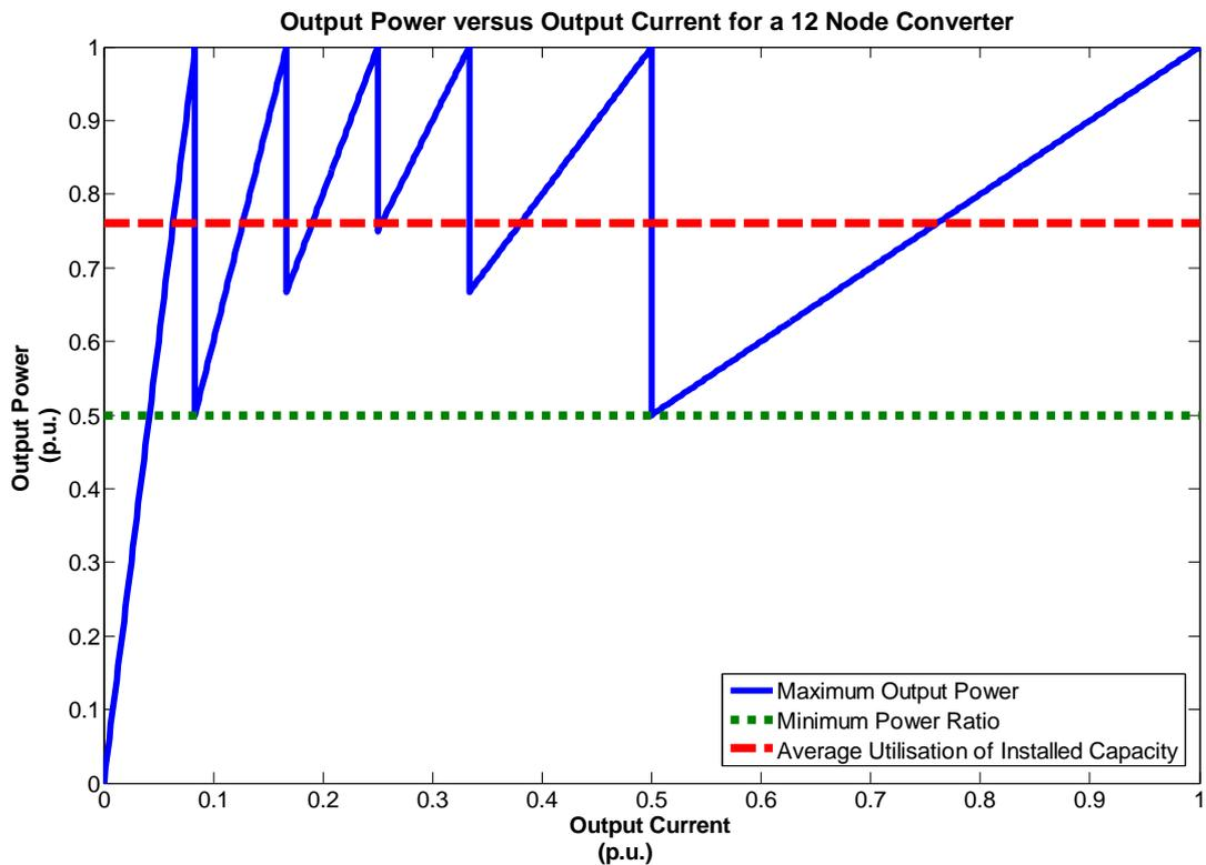
**Figure 2.4: Output power versus output current for a 12 node converter**
