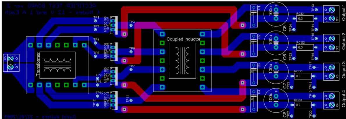
Figure 4.19: The multi-node converter secondary board's layout
