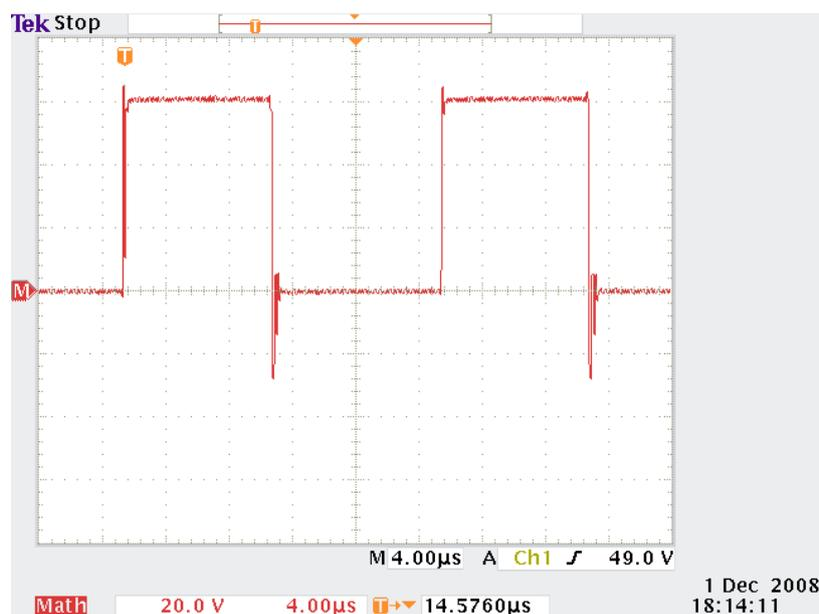
**Figure 4.10: Output into a  $100\ \Omega$  load**
