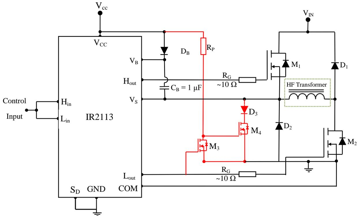
**Figure 4.6: The final high- and low-side driver schematic**
