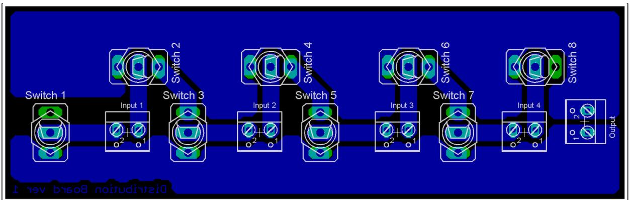
Figure B.8: Distribution board PCB layout
