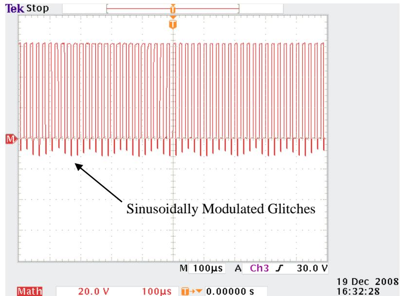
Figure 4.11: Output into a 100  $\Omega$  load
