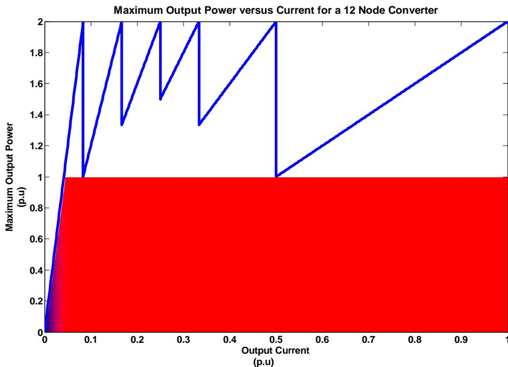
Figure 2.3: Maximum output power versus output current for a 12 node converter
