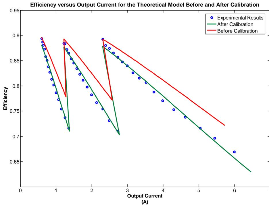
Figure 5.7: Efficiency versus output current before and after calibrating the converter.
