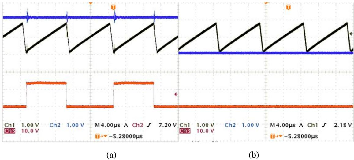
Figure A.6: The controller's ramp, control and output voltages at the maximum (a) and minimum (b) duty cycles.
