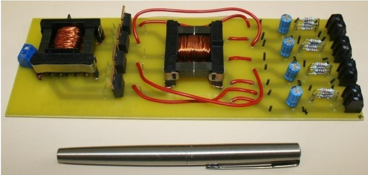
**Figure 4.20: The multi-node converter secondary prototype**
