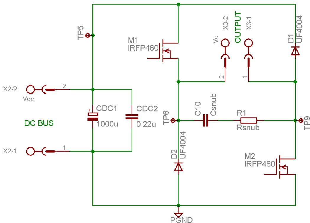
Figure B.1: Power stage schematic
