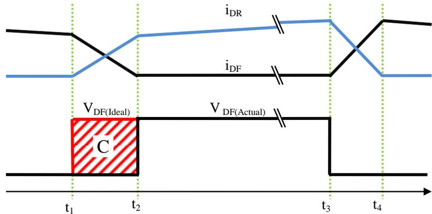
**Figure 3.4: Voltage and current waveforms for the single phase forward converter model**
