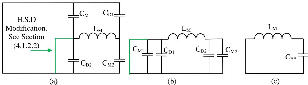
**Figure 4.13: A simplified equivalent LC circuit for the two-switch forward converter once the clamping diodes have turned off**
