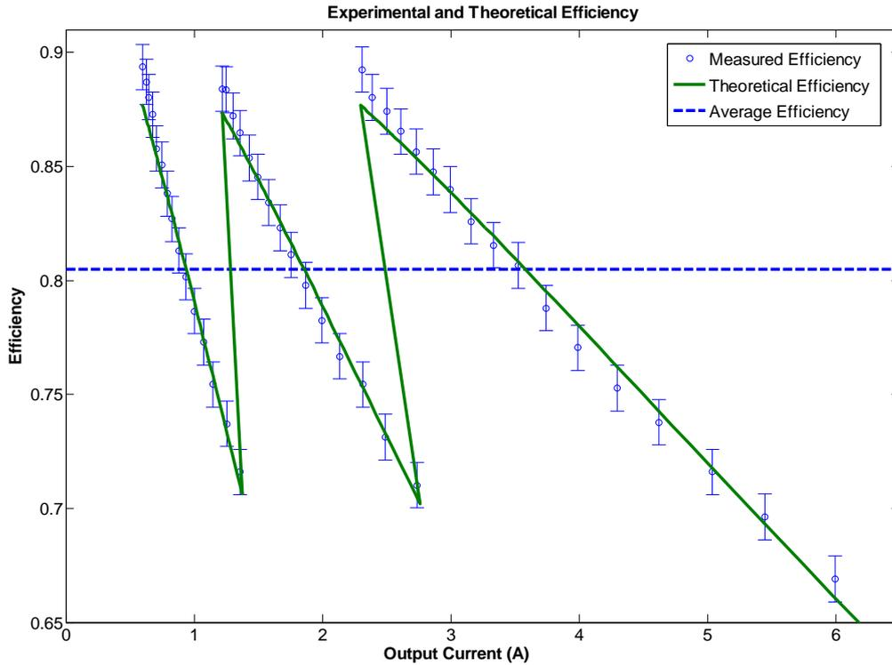
**Figure 5.6: Experimental and theoretical converter efficiency**
