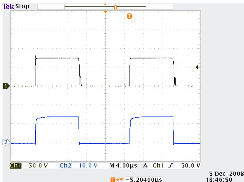
Figure A.7: MOSFET driver outputs (high-side on top)
