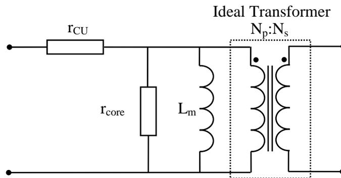
Figure 3.11: Transformer model
