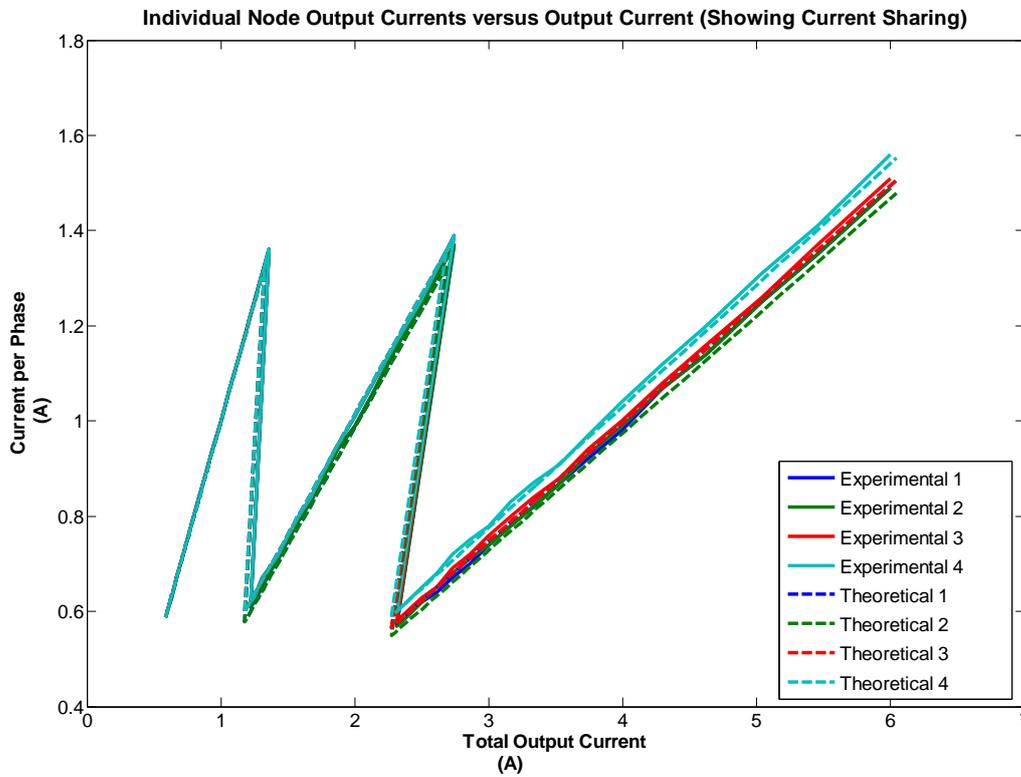
Figure 5.5: Individual node output currents versus converter output current showing current sharing
