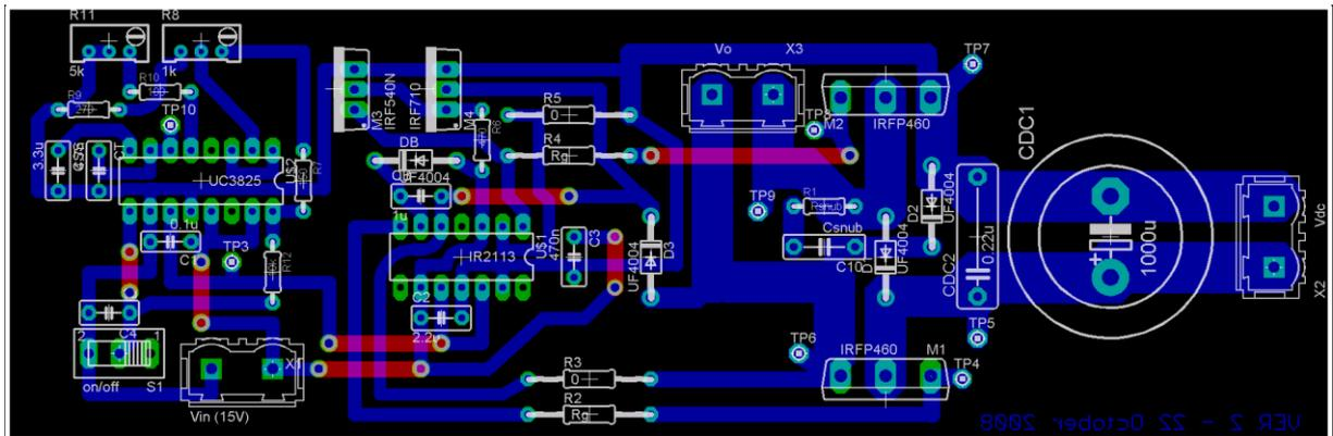
**Figure B.4: PCB layout for the converter test platform**
