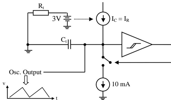
**Figure A.3:** Oscillator schematic [25]
