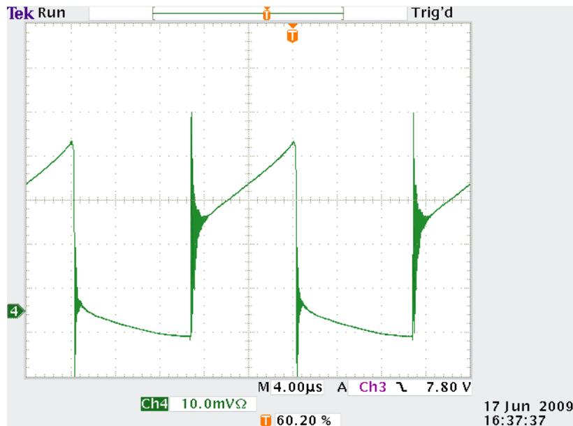
**Figure 4.16: The transformer's primary current (200 mA/div)**
