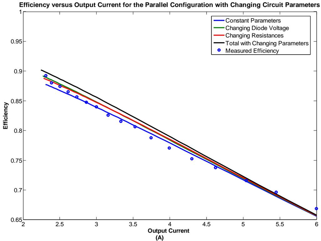
Figure 5.9: Predicted efficiency curves with changing circuit parameters
