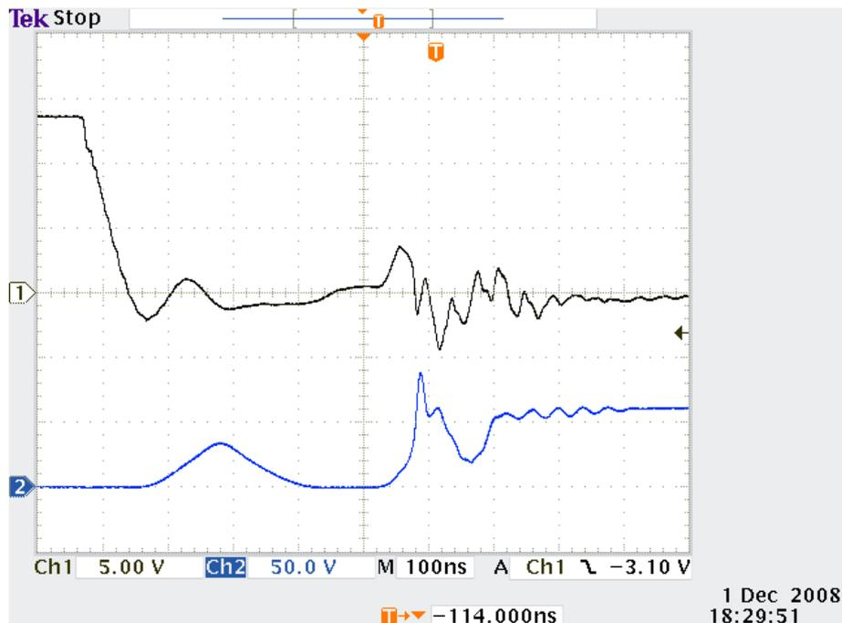
Figure A.12: Fall times for the high-side MOSFET gate and drain source voltages
