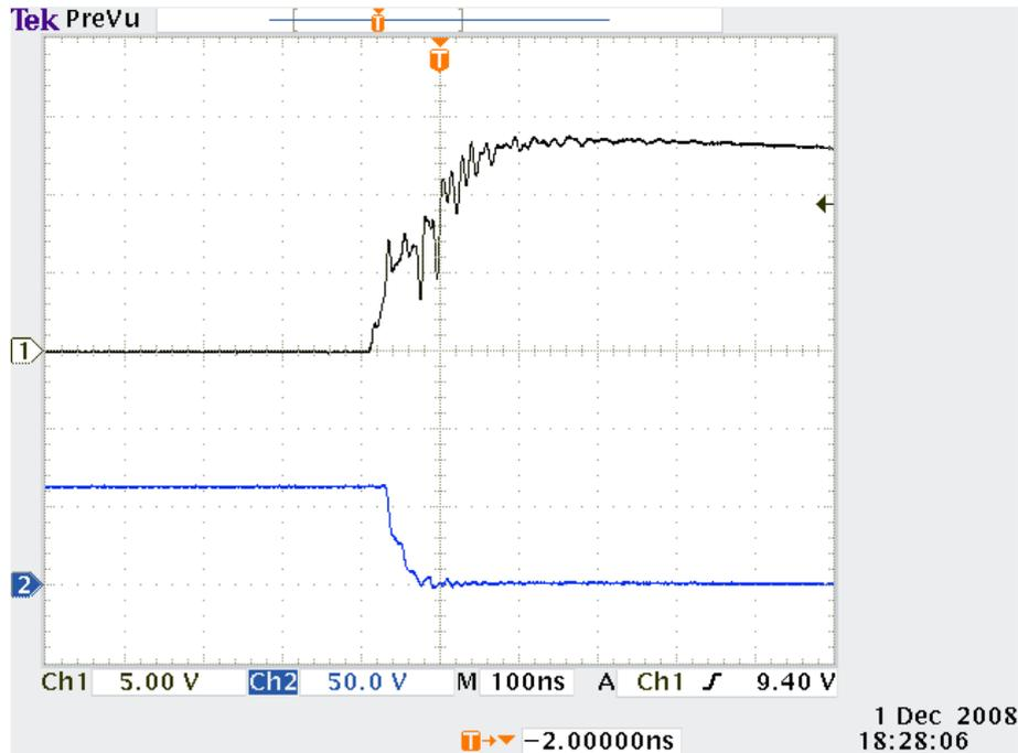
Figure A.11: Rise and fall times for the high-side MOSFET gate and drain-source voltages
