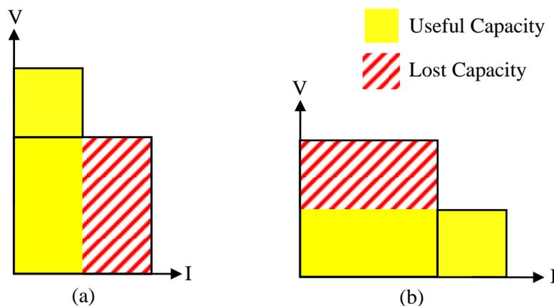
**Figure 2.5: Lost capacity with non-identical nodes. (a) Current capacity is lost when a node with a lower current capability is connected in series. (b) Voltage capacity is lost when a node with a lower voltage capability is connected in parallel.**
