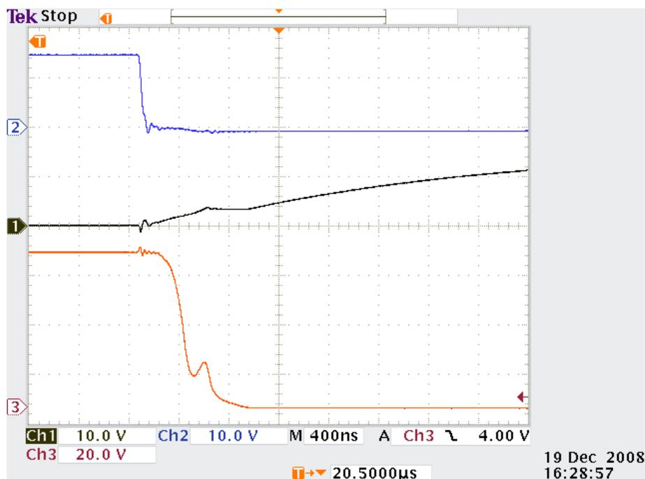
Figure A.8: Operation of the modifications made to the high-side driver
