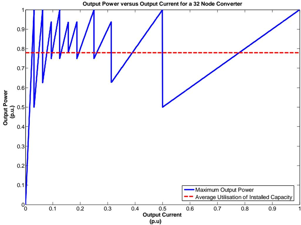
Figure 2.8: Output power versus output current for a 32 node converter
