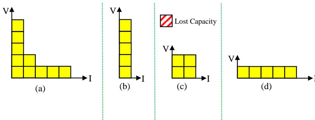
**Figure 2.7:** (a) The V-I curve for a converter with five identical nodes. (b) Serially connected nodes. (c) Nodes connected in a series/parallel combination. (d) Nodes connected in parallel.
