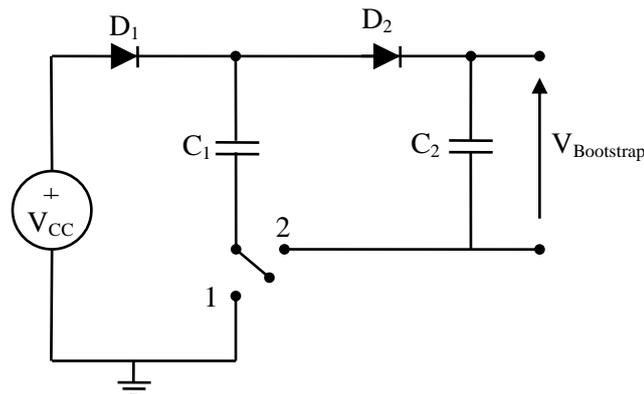
Figure 4.5: Charge pump supply schematic
