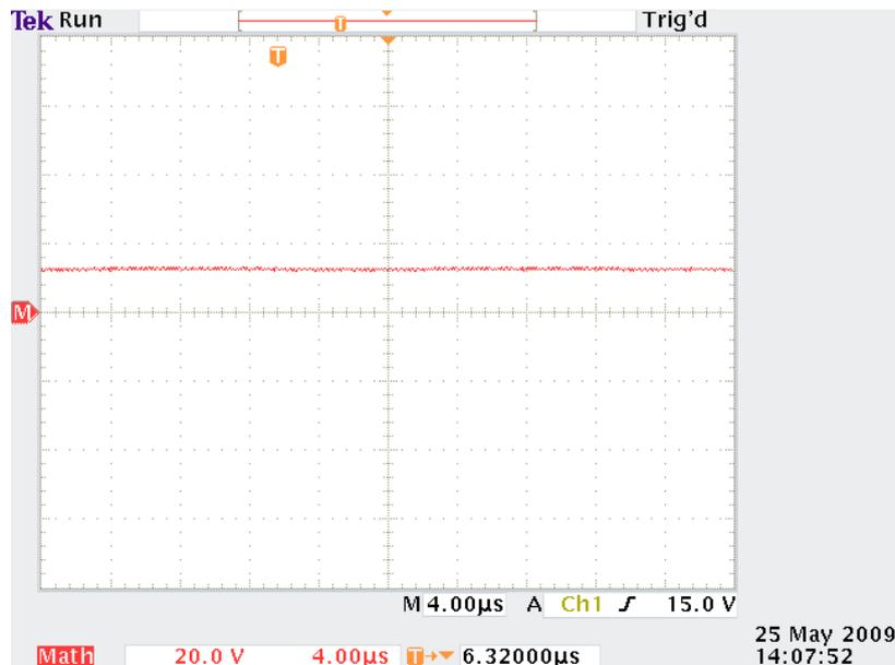
**Figure 4.24: One converter secondaries output voltage**
