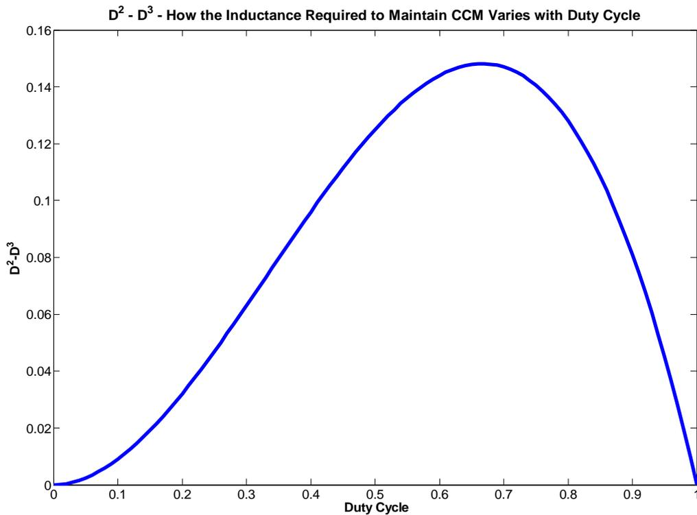
**Figure 3.7: Required filter inductance versus duty cycle**
