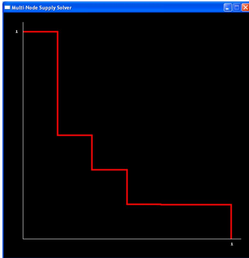
Figure 2.13: The multi-node converter simulator output showing the V-I curve for the fittest genome found for a six node converter. (The vertical axis is voltage p.u. and the horizontal axis is current p.u.)
