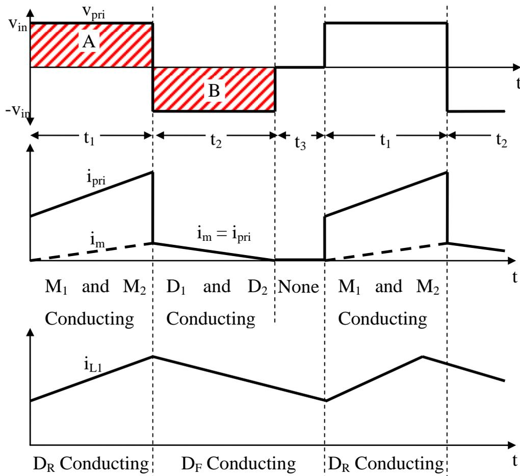
Figure 3.2: Ideal voltage and current waveforms for the two-switch forward converter
