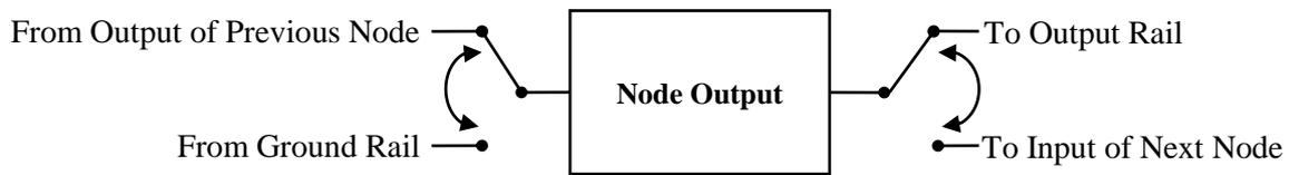
Figure 4.25: The sub-circuit schematic
