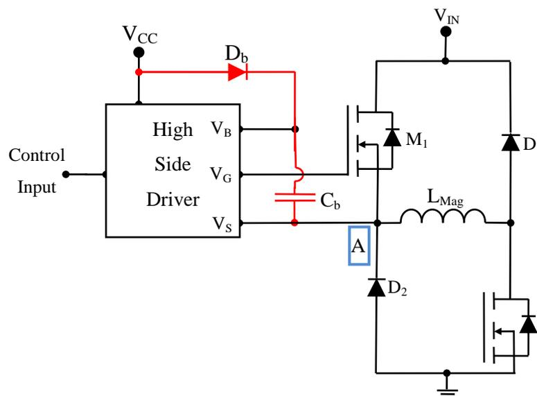
**Figure 4.4: Bootstrap capacitor operation with a two-switch forward converter**
