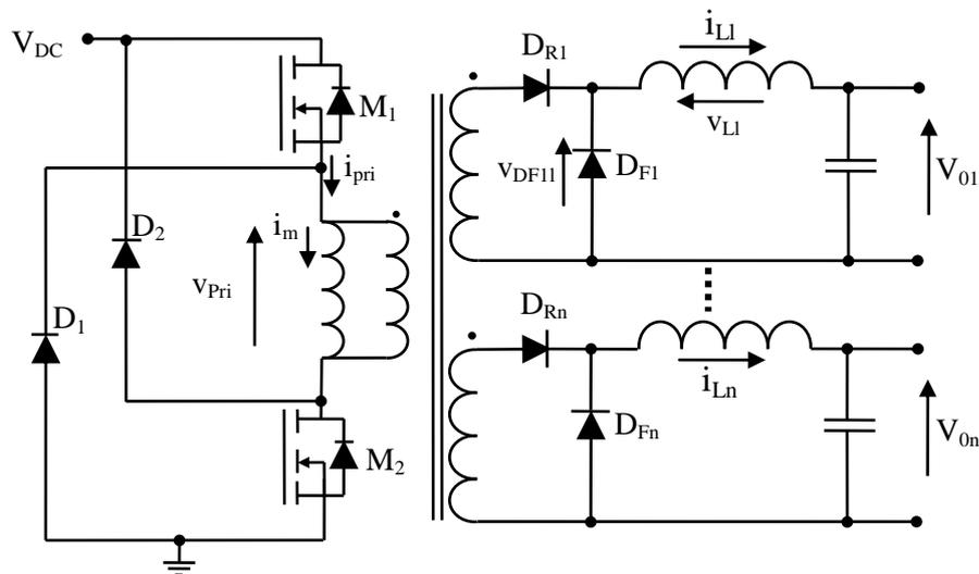
Figure 3.8: The two-switch forward converter with multiple identical secondaries
