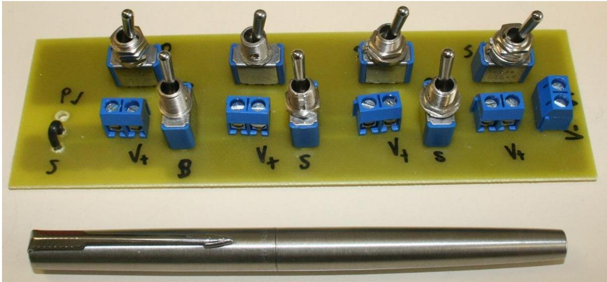
Figure 4.27: The prototype distribution board
