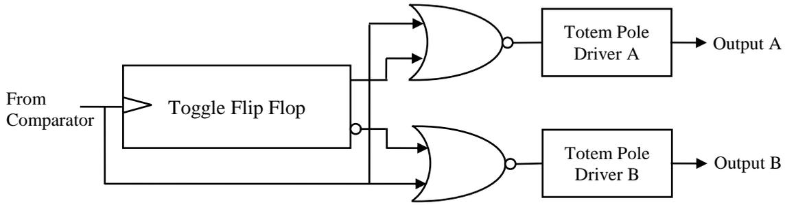
**Figure A.4: Output stage schematic [25]**
