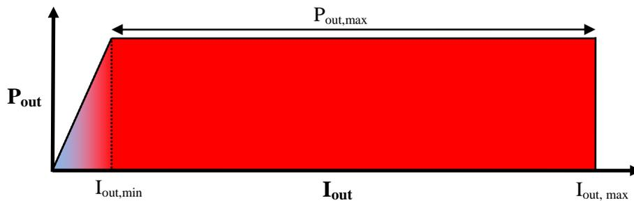
**Figure 1.4: Constant maximum output power over a wide range**
