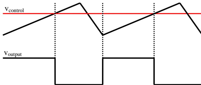
**Figure A.1: Generation of PWM using a triangular waveform and a comparator**
