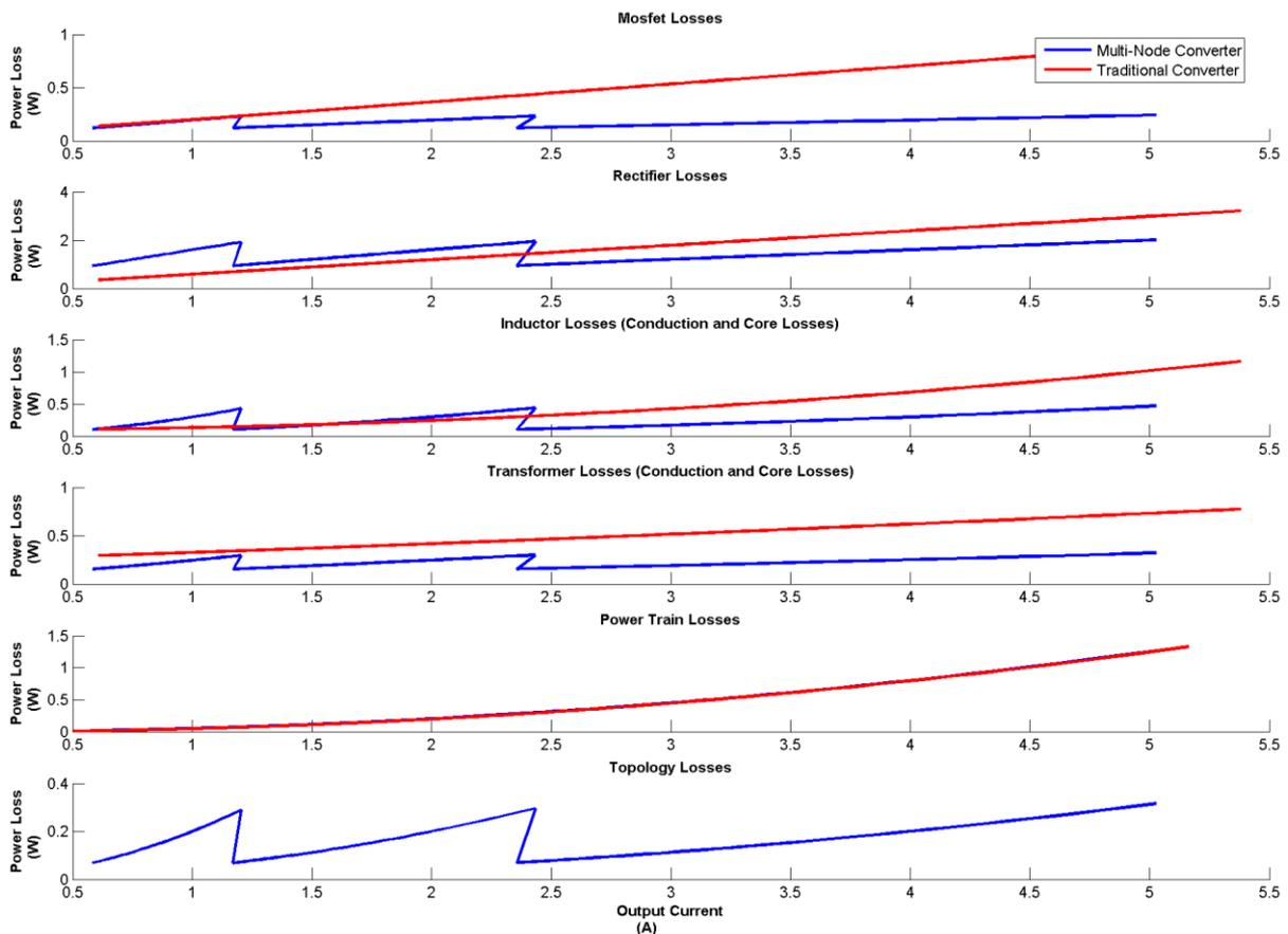
Figure 3.14: Component losses for both converters
