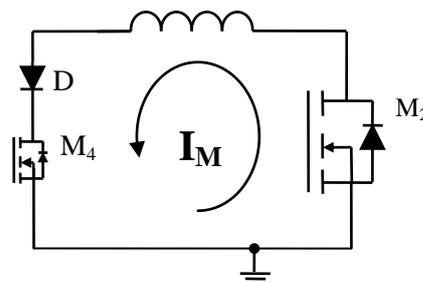
Figure 4.14: Equivalent circuit when the oscillation ends
