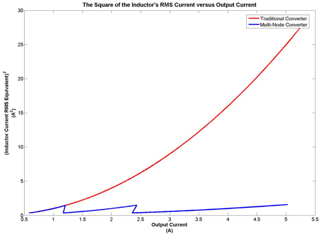
**Figure 3.15: RMS inductor current squared over the output range**
