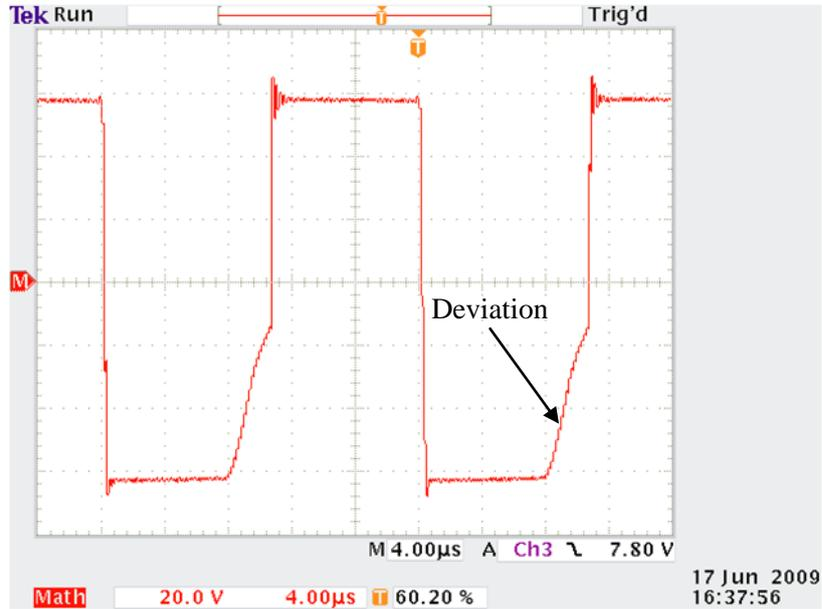
**Figure 4.12: The forward converter test platform’s output into a transformer load**
