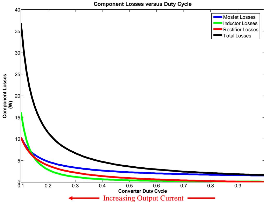
Figure 1.6: Component losses versus duty cycle
