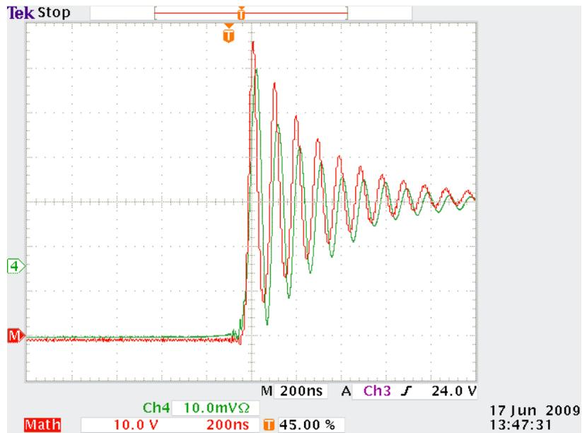
**Figure 4.23: Transformer primary current (green at 200 mA/div) and rectifier output oscillation (red)**
