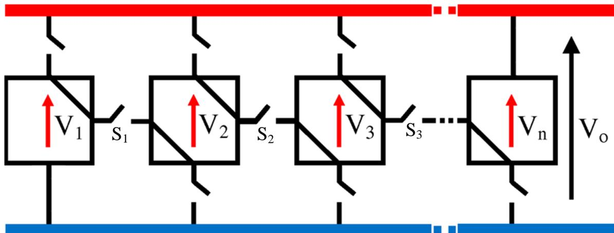
Figure 2.1: The multi-node converter schematic with the switches numbered
