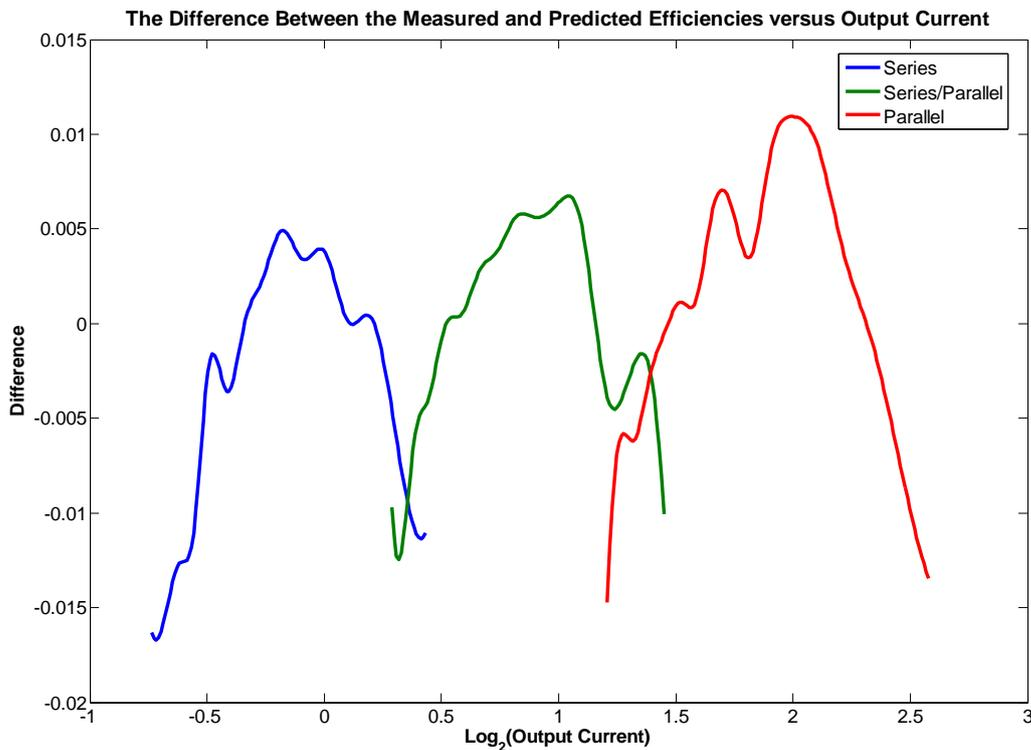
**Figure 5.8: The difference between the experimentally measured and theoretically predicted efficiencies versus  $\log_2(I_o)$**
