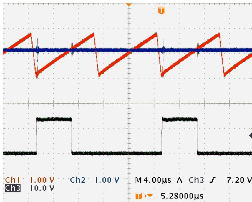
Figure A.5: PWM ramp and control voltages with the resultant controller output
