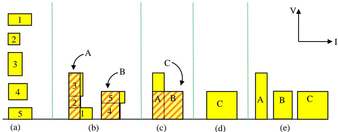
**Figure 2.9:** (a) The individual V-I curves for the 5 nodes. (b) The nodes are combined into node strings consisting of one or more nodes depending on which switches are closed. The V-I curves are combined accordingly. (c) The node strings then combined to get the final V-I curve for this configuration. (d) The final V-I curve for the configuration. (e) the V-I curves that are saved for these nodes with the given switch position
