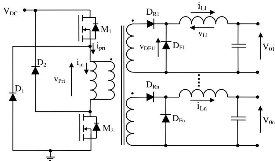
**Figure 3.1: The two-switch forward converter with multiple identical secondaries**
