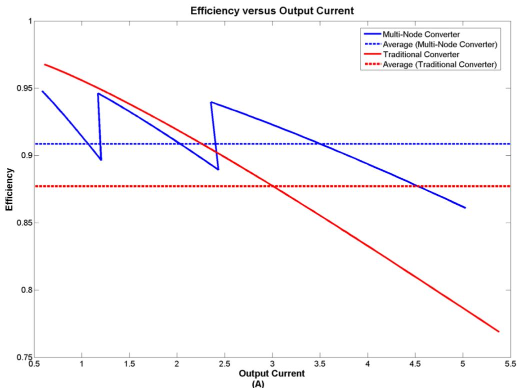
Figure 3.16: Efficiency versus output current for both converters
