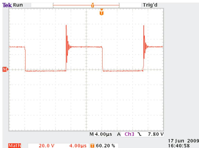
**Figure 4.22: The rectifier's output voltage**
