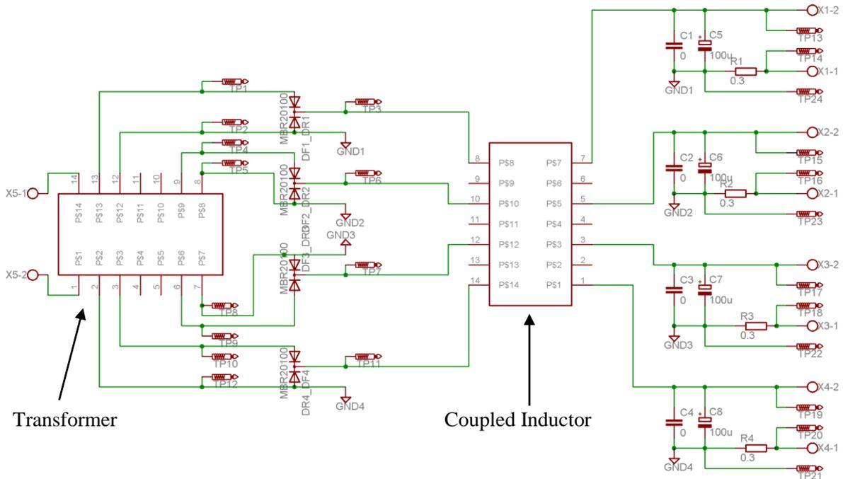
Figure B.5: Multi-node secondary schematic
