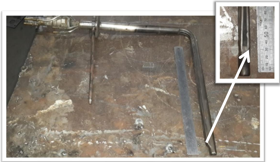
Figure 2-8:LC-4 Isokinetic PF Sampling Nozzle
