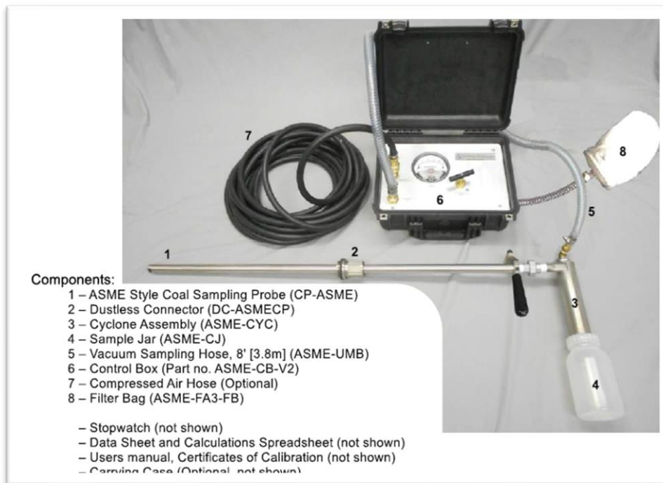
Figure 2-15: ASME PTC 4.2 Coal Sampler (Airflow Sciences Equipment, 2021)
