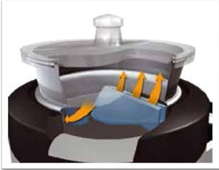
Figure 2-19: Air Jet Sieving (RETSCHE GmbH., 2019)
