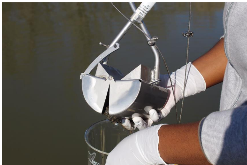
Figure 3.2 0.5 L Van Veen as used during sampling
