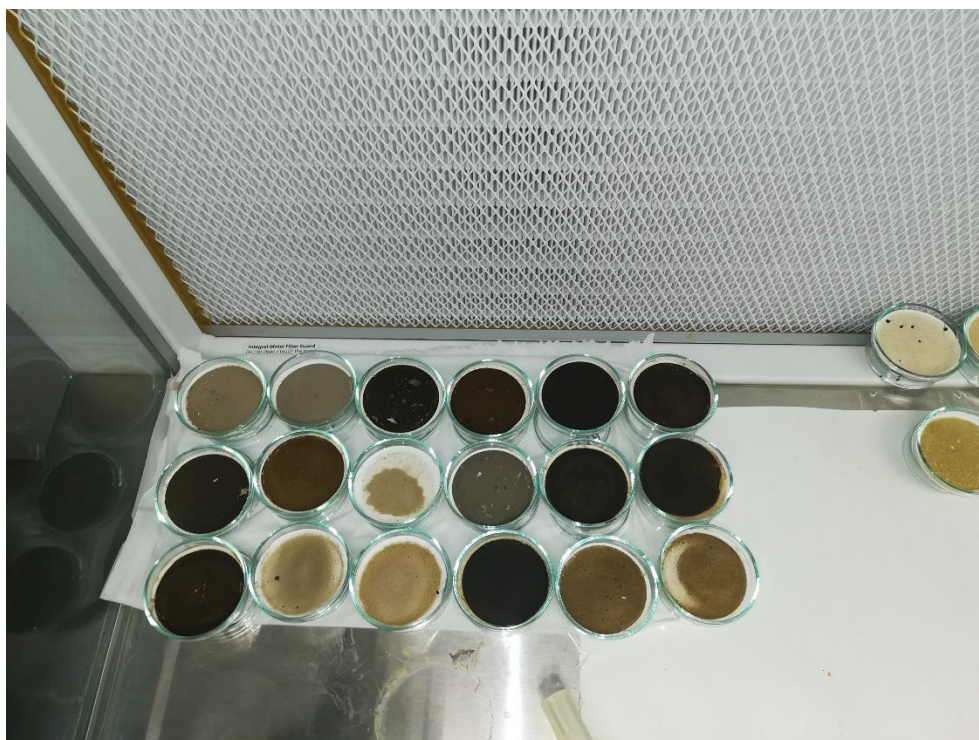
Figure 3.5 Air-drying of filter papers in the laminar flow cabinet
