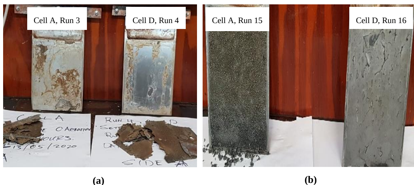
Figure 4.13 a) Characteristics of deposit from run 3 and run 4 b) Characteristics of deposit from run 15 and run 16
