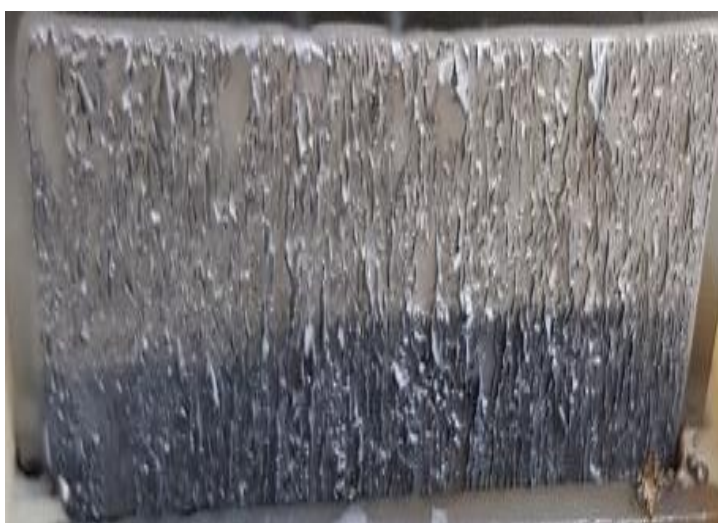
Figure D.9 Burning on the metal surface from the cathode plate (Run 9 – 10) due to the starting up of the cells at concentration below 9 mg/L
