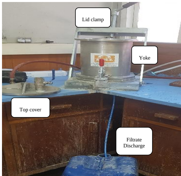
Figure 3.4 Macsalab filter press for solid separation
