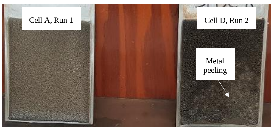
Figure 4.10 Physical characteristics of metal run 1 and run 2 before stripping
