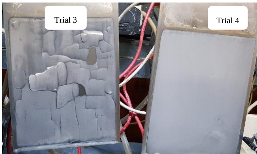
Figure C.5 Impact of buffed and unbuffered plated on the plating of trial 3 and trial 4
