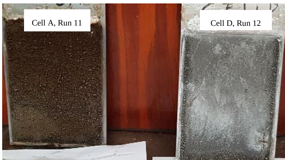
Figure 4.16 Digital images of manganese metal produced in run 11 and run 12
