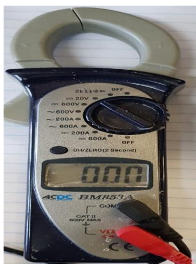
Figure B.1 Ammeter for voltage and current measurement
