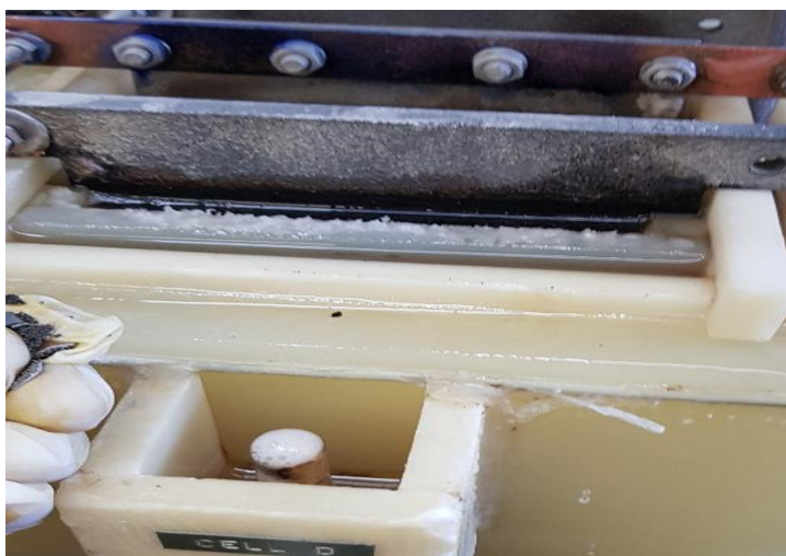
Figure D.7 Anolyte blockage at the overflow weir due to the presence of \text{Mn}(\text{OH})_2 in the pipeline. Mn metal flakes used to unblock the weir by metal dissolution with the anolyte
