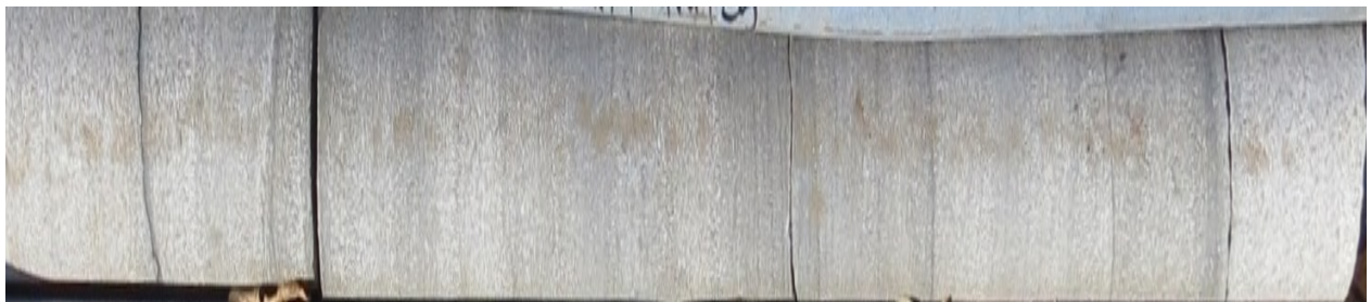
Figure 18: Medium-grained sandstone with lower angle horizontal stratification (source: NG-108).
