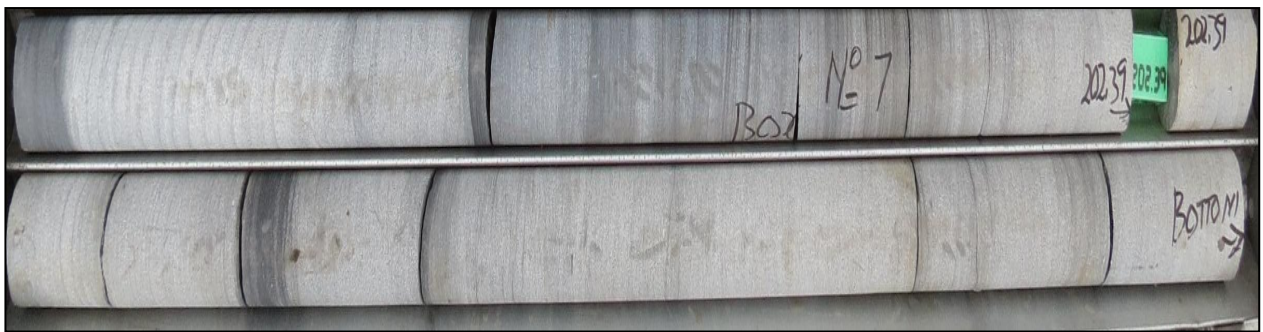
Figure 17: Coarse-grained, cross-laminated, whitish sandstone in drill hole NG-108.
