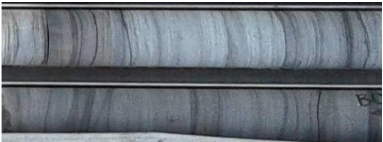
Figure 13: Medium-grained sandstone with interbeds of laminated siltstone in drill hole NG-108 (an example of unit 2 and some part of unit 11 of the ZAC stratigraphy).
