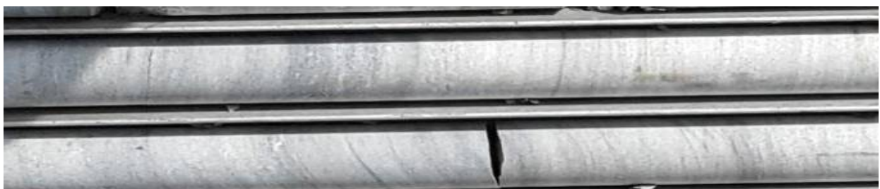
Figure 14: Medium- to coarse-grained sandstone in drill hole NG-108 (an example of unit 3, unit 5, unit 7, and unit 9 of the general stratigraphy of ZAC).
