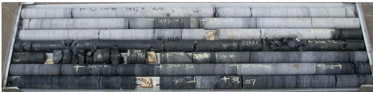
Figure 7: A photograph of a drill core from a drill hole NG-108 located 300m from Section 30 showing the roof, Main Seam, and floor of the Main Seam.
