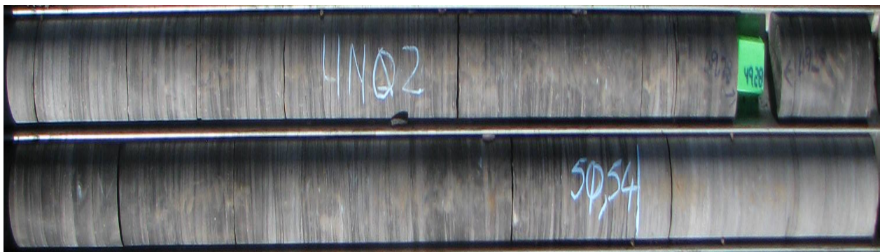
Figure 19: Fine-grained siltstone interlaminated with shale in drill hole NG-108.
