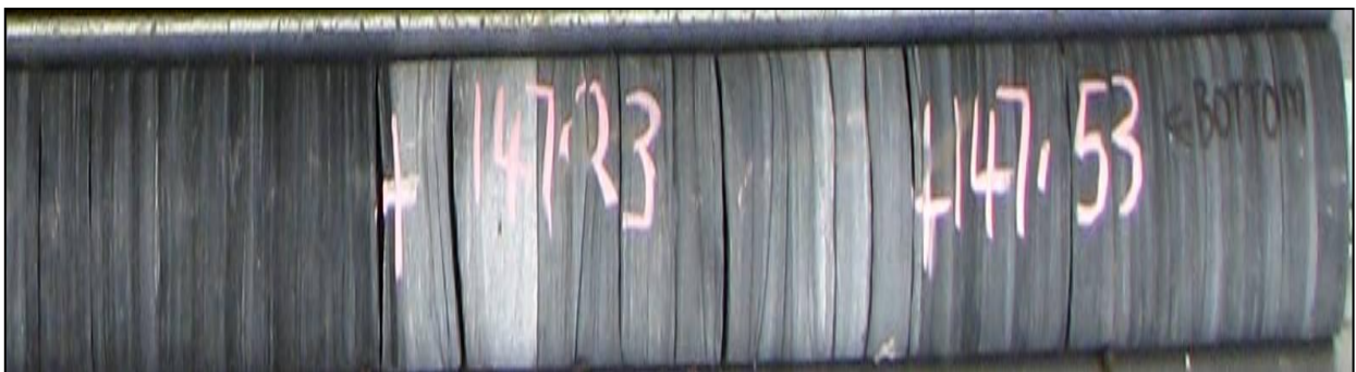
Figure 16: Very fine-grained sandstone interbedded with shale and siltstone in drill hole NG-108.
