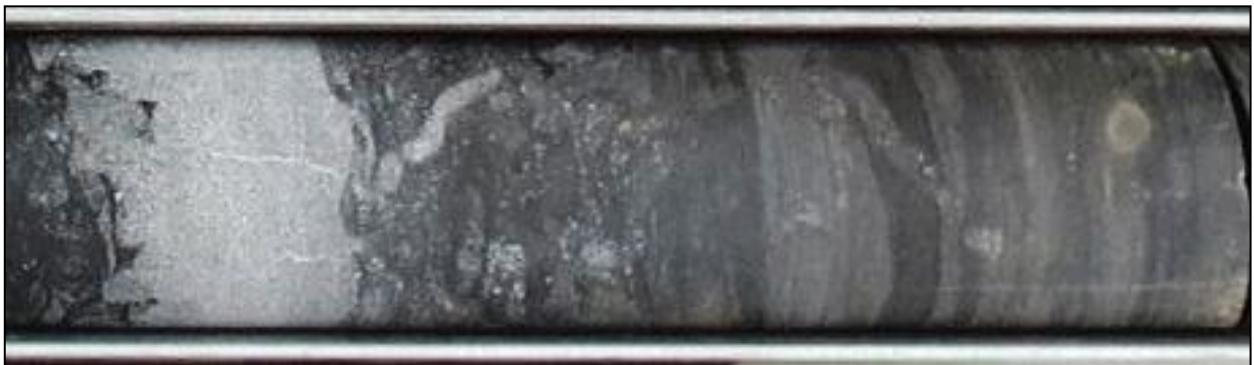
Figure 15: Coarse-grained sandstone interlaminated with shale in drill hole NG-108, showing vertical bioturbation burrows.
