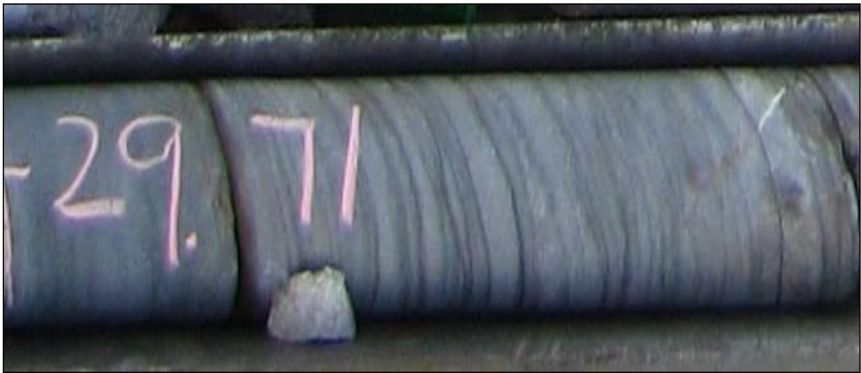
Figure 12: Wave-ripple cross-lamination in drill hole NG-108 (an example of unit 1 of the ZAC stratigraphy).
