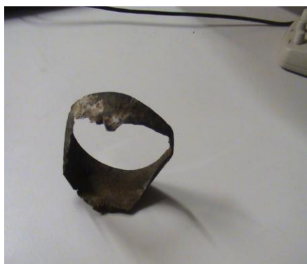
Figure 4.40. Section of the original lance from Tsumeb smelter.
