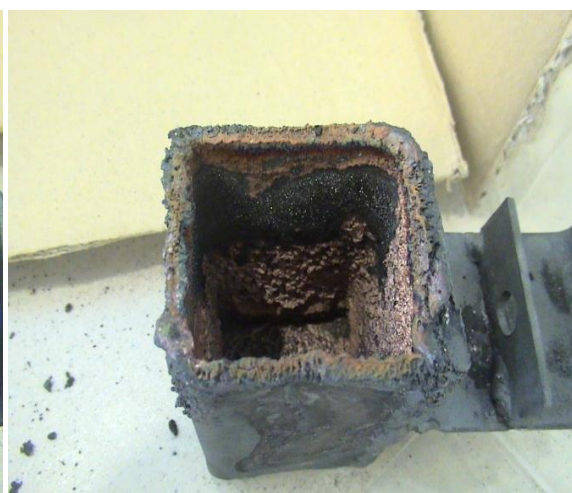
Figure 4.2. Photograph showing the interior of crucible treated for 40 minutes in inert conditions without agitation.
