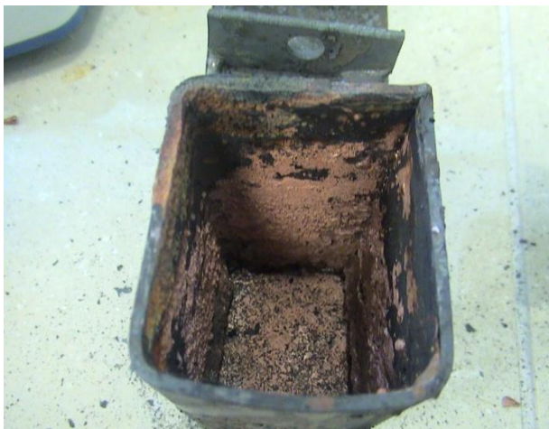
Figure 4.7. Photograph showing the interior of crucible treated 100 minutes in inert conditions without agitation.
