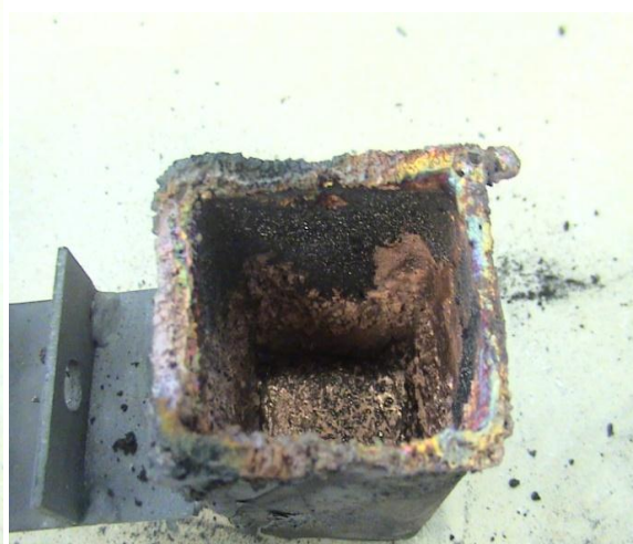
Figure 4.4. Photograph showing the interior of crucible treated for 80 minutes in inert conditions without agitation.
