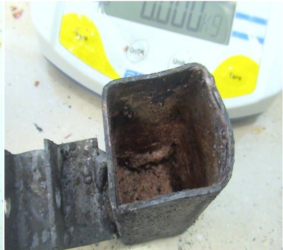
Figure 4.6. Photograph showing the interior of crucible treated for 80 minutes in inert conditions with agitation.
