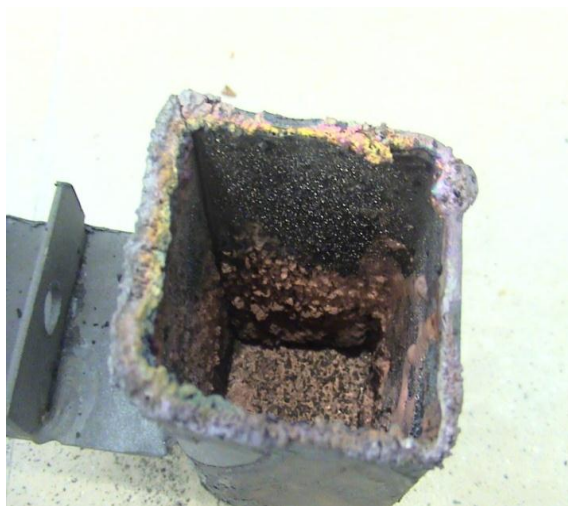
Figure 4.3. Photograph showing the interior of crucible treated for 20 minutes in inert conditions without agitation.
