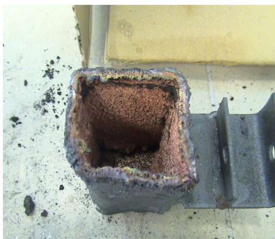
Figure 4.1. Photograph showing the interior of crucible treated for 60 minutes in inert conditions without agitation.
