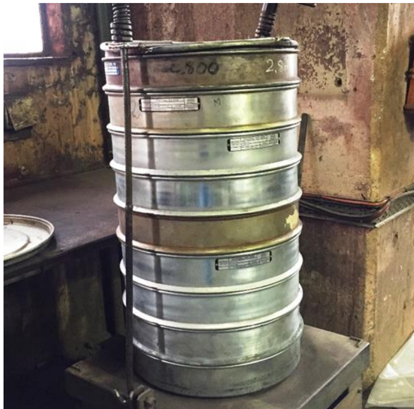
Figure 7 – Mechanical Screening Equipment (Exxaro)
