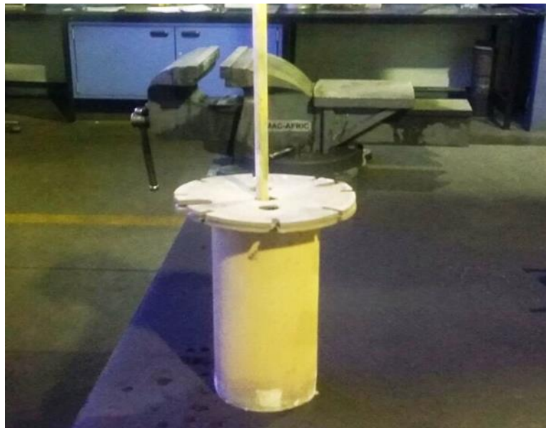
Figure 8 – Coal Holder (Bureau Veritas, Lab Scale)
