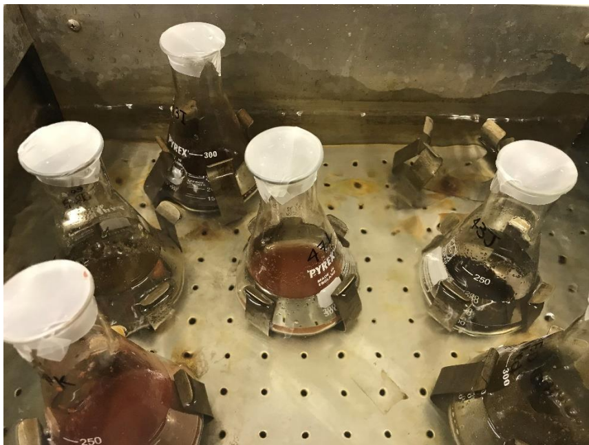
Figure 3.11. A picture of the shaking bath and Erlenmeyer flasks containing the leach slurries.
