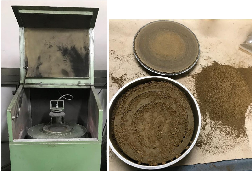
Figure 0.2. Picture of the Sieb Technik Mill and a sample bowl with the ZKD ore.
