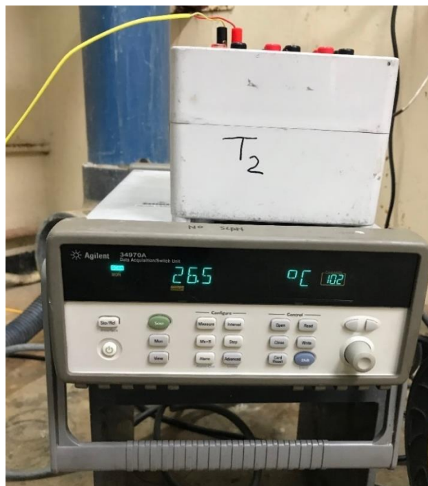
Figure 0.7. Data logger used to monitor the sample bed temperature through the K-type thermocouple.
