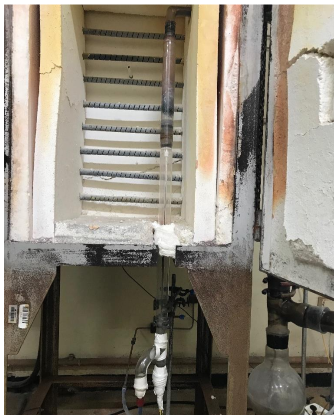
Figure 3.10. A picture of the sulfation roasting experiments furnace and reactor setup.
