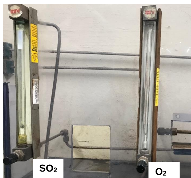
Figure 3.4. Picture of the ¼’’ NPTF rotameters used for the sulfation roasting experiments.
