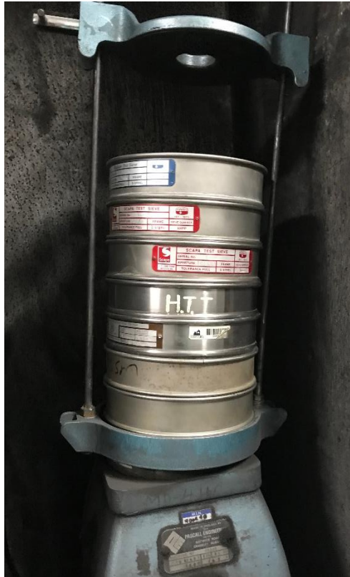
Figure 0.4. A picture of the vibrating sieve shaker and woven wire sieves used for the sizing of the samples.
