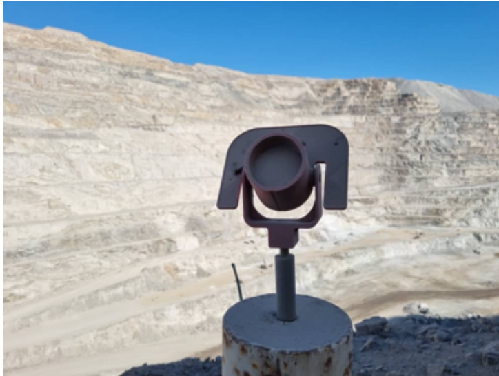
Figure 4-21: Prism 229 fully covered in dust on the date of recovery (Aero Vision Drone Services, 2022).
