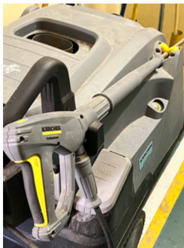
Figure 3-8: A Kärcher Professional 1.170-902.0 HDS 6/14 CX hot water High-Pressure washer.
