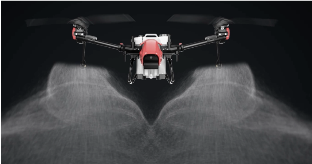
Figure 4-29: An XAG V40 Agricultural Drone with an activated RevoSpraying System (XAG, 2022b).
