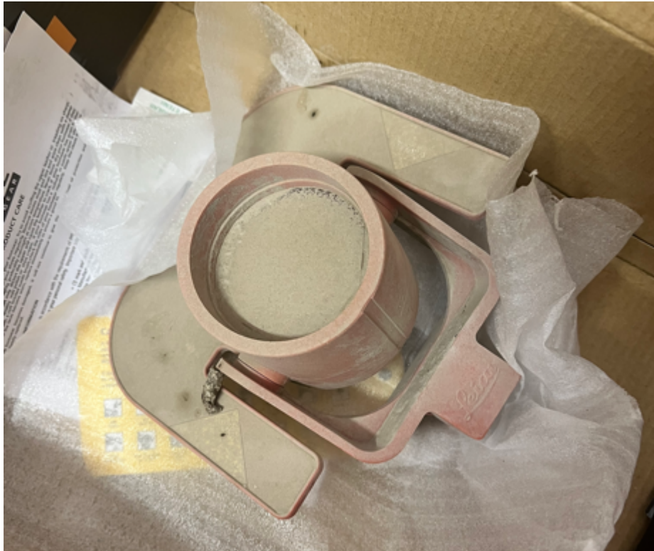
Figure 4-22: The dust accumulation on Prism 229.
