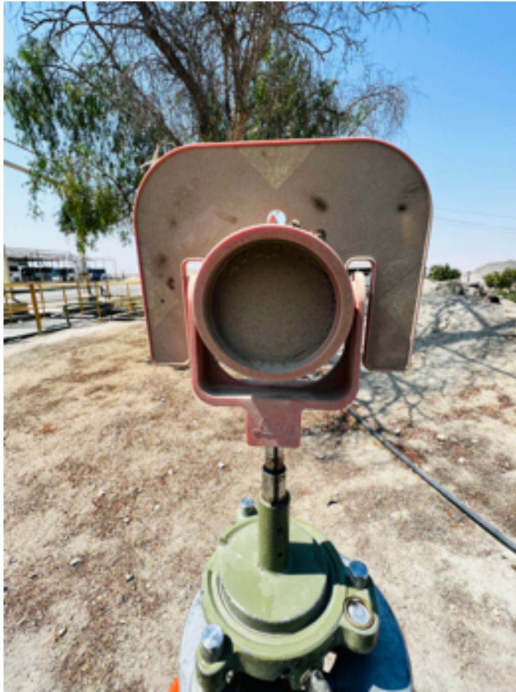
Figure 3-10: Recovered Prism 229 mounted on a tripod for the cleaning experiment.
