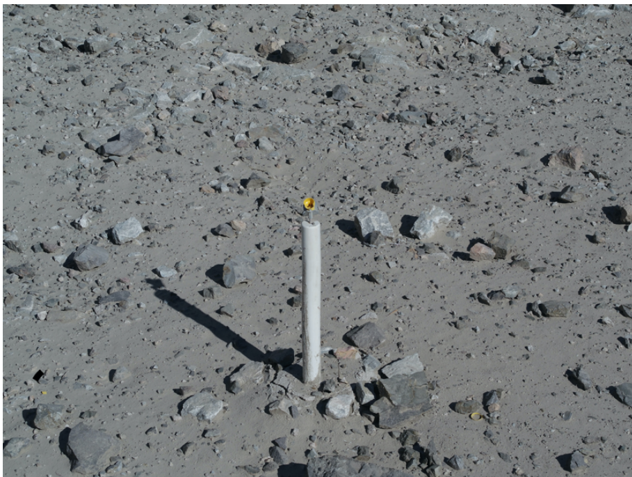
Figure 4-19: A prism with a missing glass surface (RUL Internal Data, 2022).
