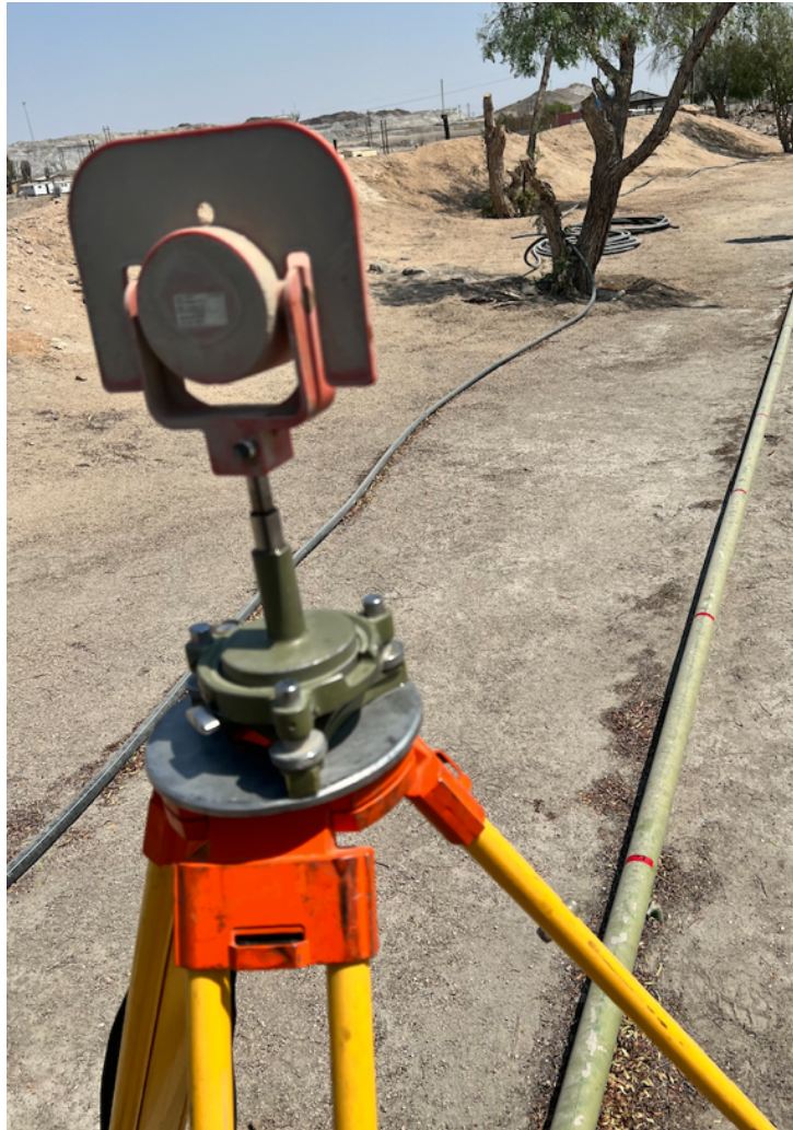
Figure 3-11: Distances from the prism marked out at 1-metre intervals.
