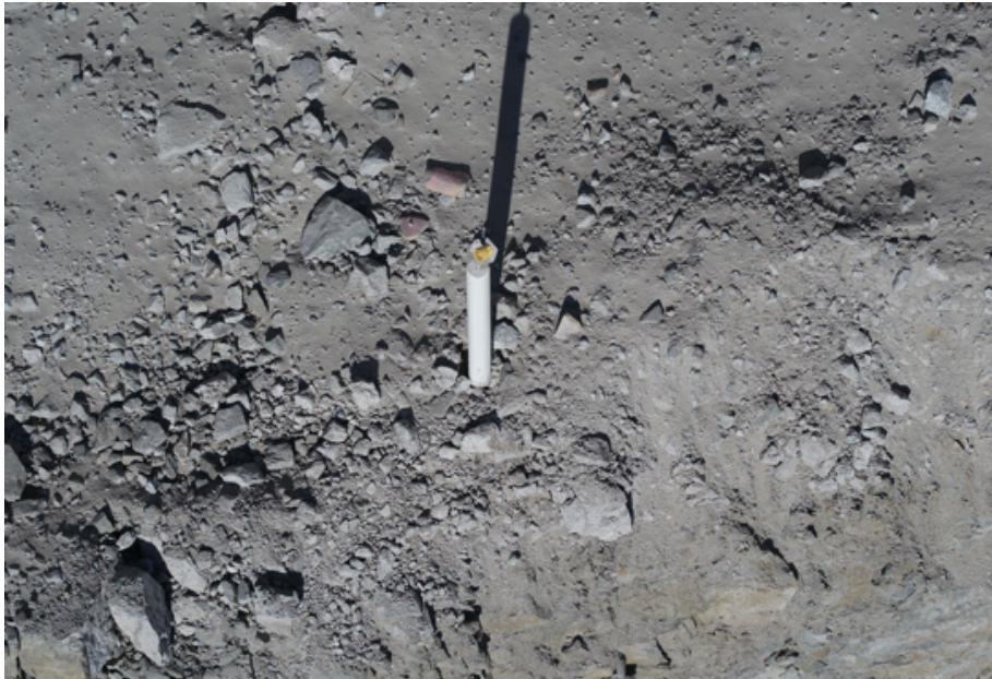
Figure 1-1: A prism installed at an open edge (highwall) (RUL Internal Data, 2022).
