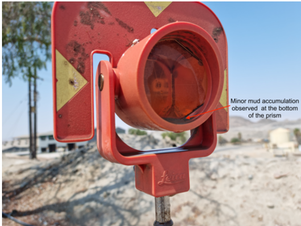
Figure 5-9: Initial outcomes of the spray cleaning experiment (Type: Leica GPR111).
