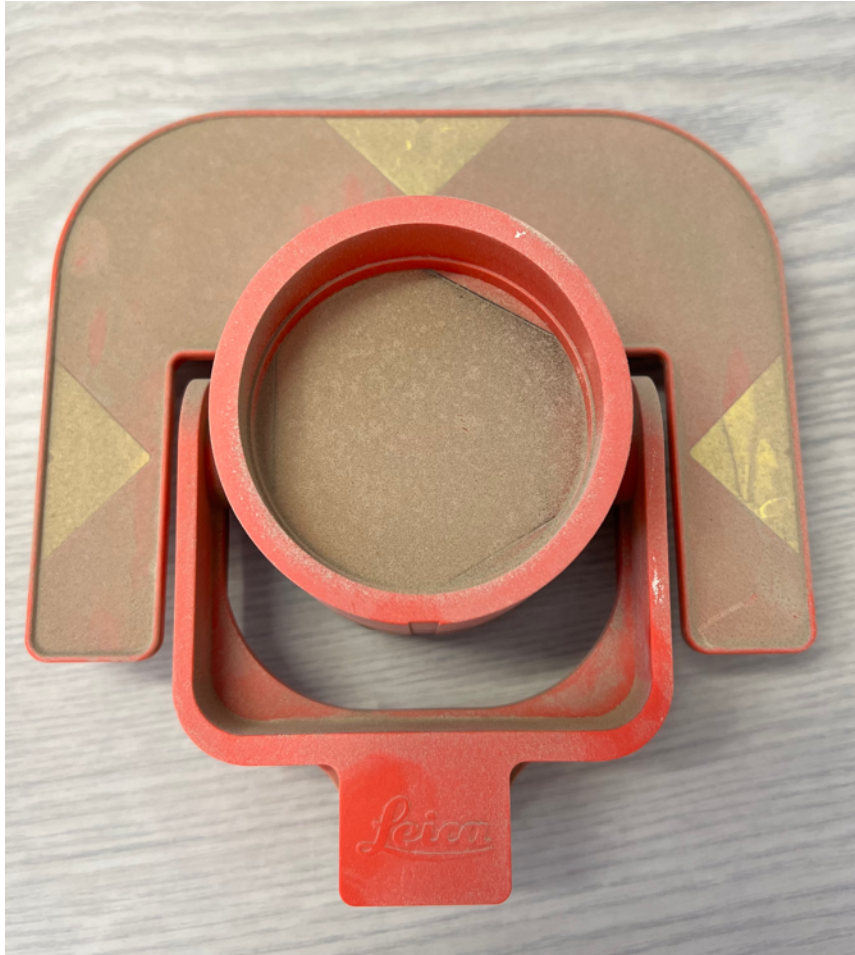
Figure 5-8: Dust accumulation on the newly installed prism.
