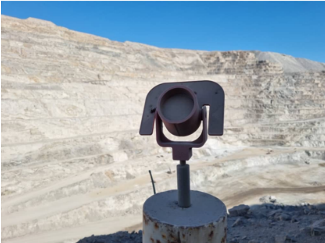
Figure 1-4: A monitoring Prism 229 covered with dust.
