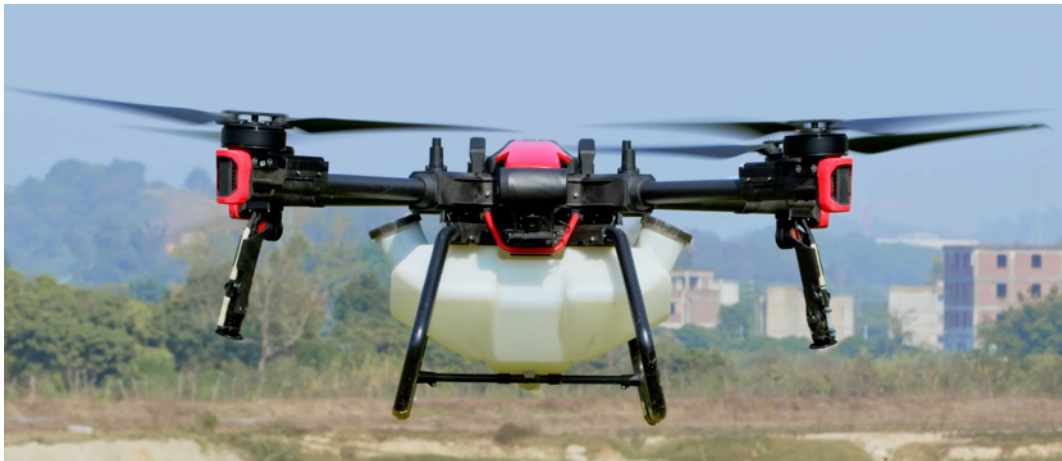
Figure 4-26: An XAG P100 Agricultural Drone fitted with a sprayer tank (2) (XAG, 2022a).
