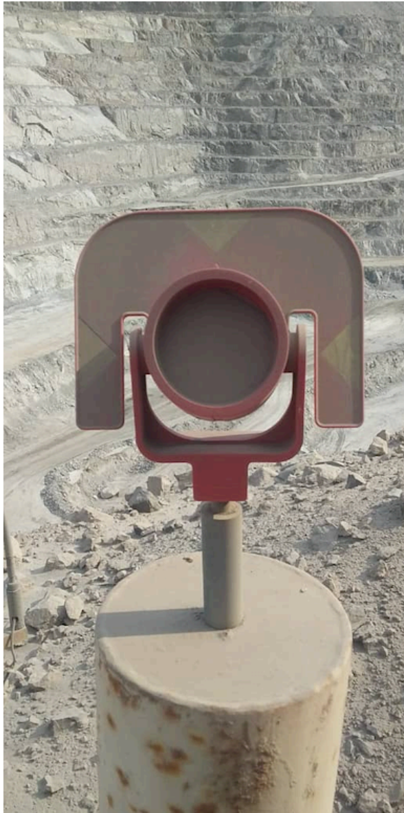
Figure 3-7: The dust coverage on the test prism (Type: Leica GPR111) two months after installation (Aero Vision Drone Services, 2022).
