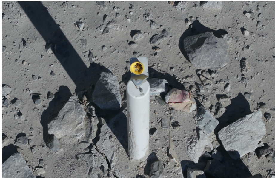
Figure 4-16: A close-up image of a prism with a missing glass surface (RUL Internal Data, 2022).
