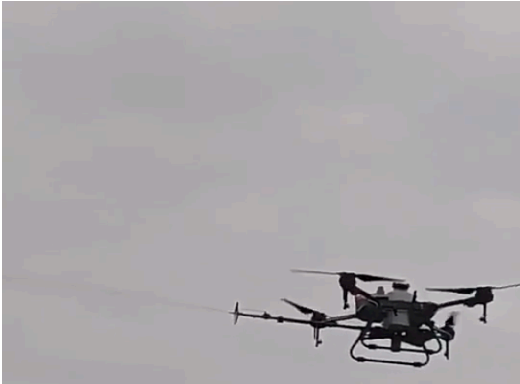
Figure 4-35: Weifang Little Stone Craft M50S Agricultural Sprayer Drone with an activated horizontal sprayer (Weifang Little Stone Craft Co., 2022).
