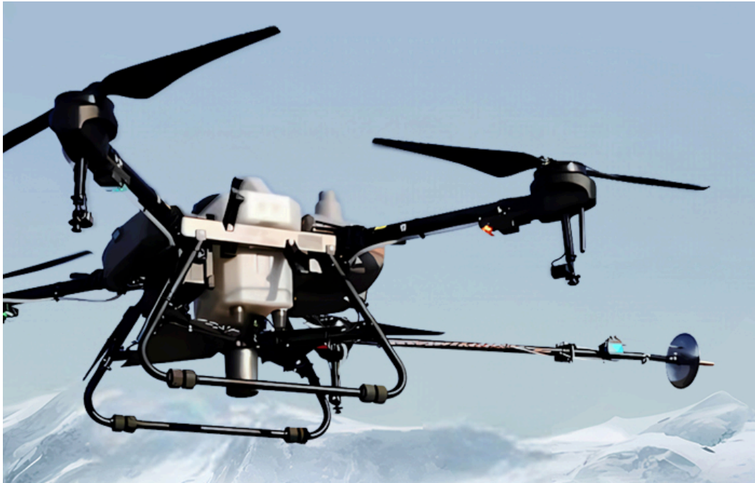
Figure 4-33: Weifang Little Stone Craft M50S Agricultural Sprayer Drone with a horizontal nozzle (Weifang Little Stone Craft Co., 2022).
