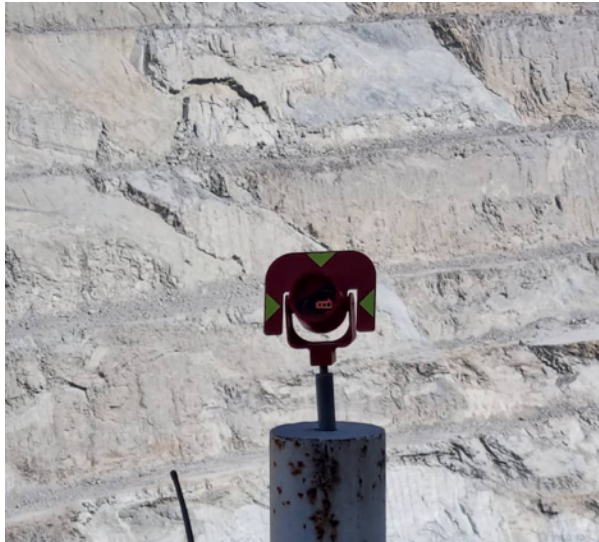
Figure 3-6: A test prism on the Installation date: 10 th of August 2022 (Aero Vision Drone Services, 2022).
