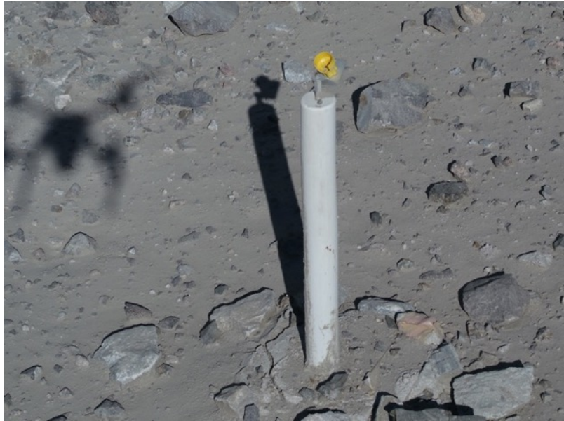
Figure 1-3: A prism-focused UAV inspection showing a damaged prism (RUL Internal Data, 2022).
