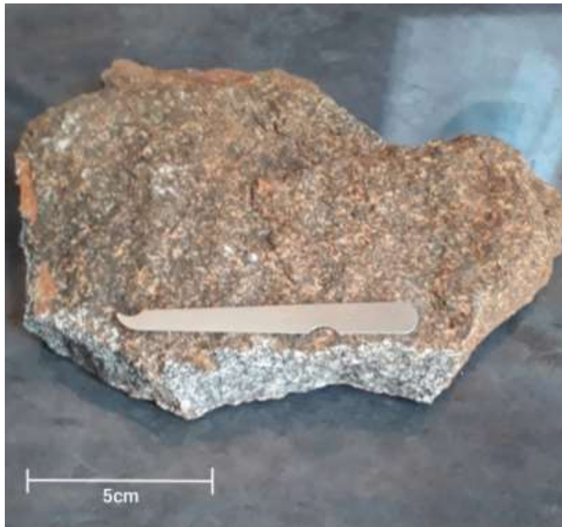
Figure 19: Metadolerite Rock Sample Collected from the Study Area
