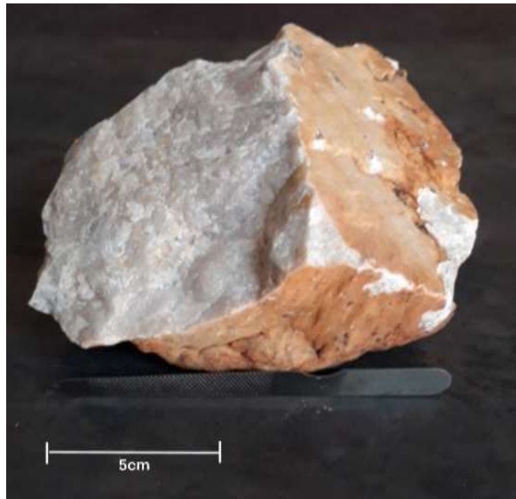
Figure 13: Quartzite Rock Sample Collected from the Study Area
