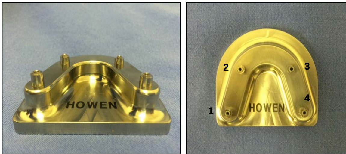
Figure 0.1 Master Model. The implant fixtures were numbered as shown on the right, to identify the distance and angle measurements.
