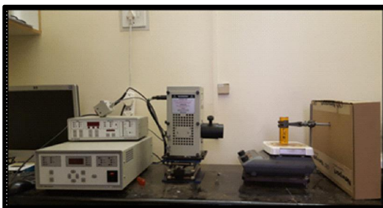
Figure 3.1: Schematic representation of the Newport Illuminator Solar Simulator Oriel Instruments WX00048 [1].
