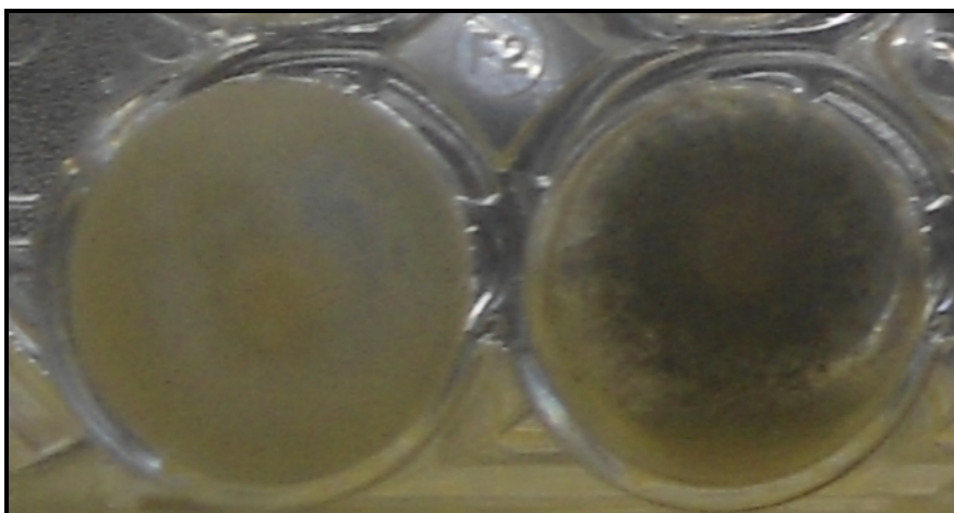
Figure 3.6: An enlarged view of two adjacent contaminated wells. Note the different kinds of coloration that indicate contamination
