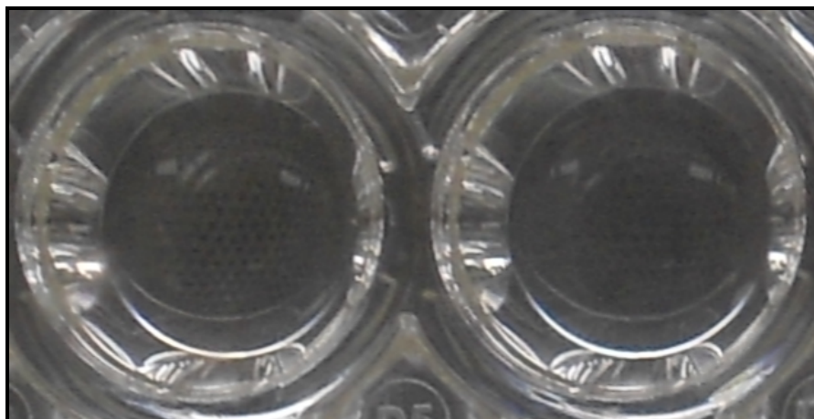
Figure 3.4: An enlarged view of two adjacent negative wells. No cloudy formation or coloration is visible. Notice the near symmetrical reflection of light visible in the left and right parts of the upper region in both wells
