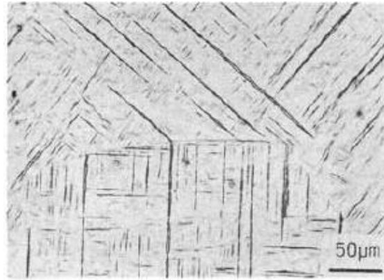
Figure 2.5: Light micrograph (LM) of acicular martensite in Ti-6Al-4V alloy quenched from the \beta phase field (Lütjering et al., 2000).
