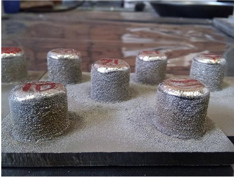
Figure 3.5: Coupon shaped samples of Ti-6Al-4V+10 wt% Mo built in the LENS ™ machine (the samples are 15 mm across and 11 mm high).
