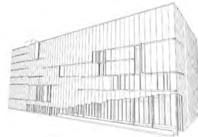
north-facing resonant skin with closed outer panels
