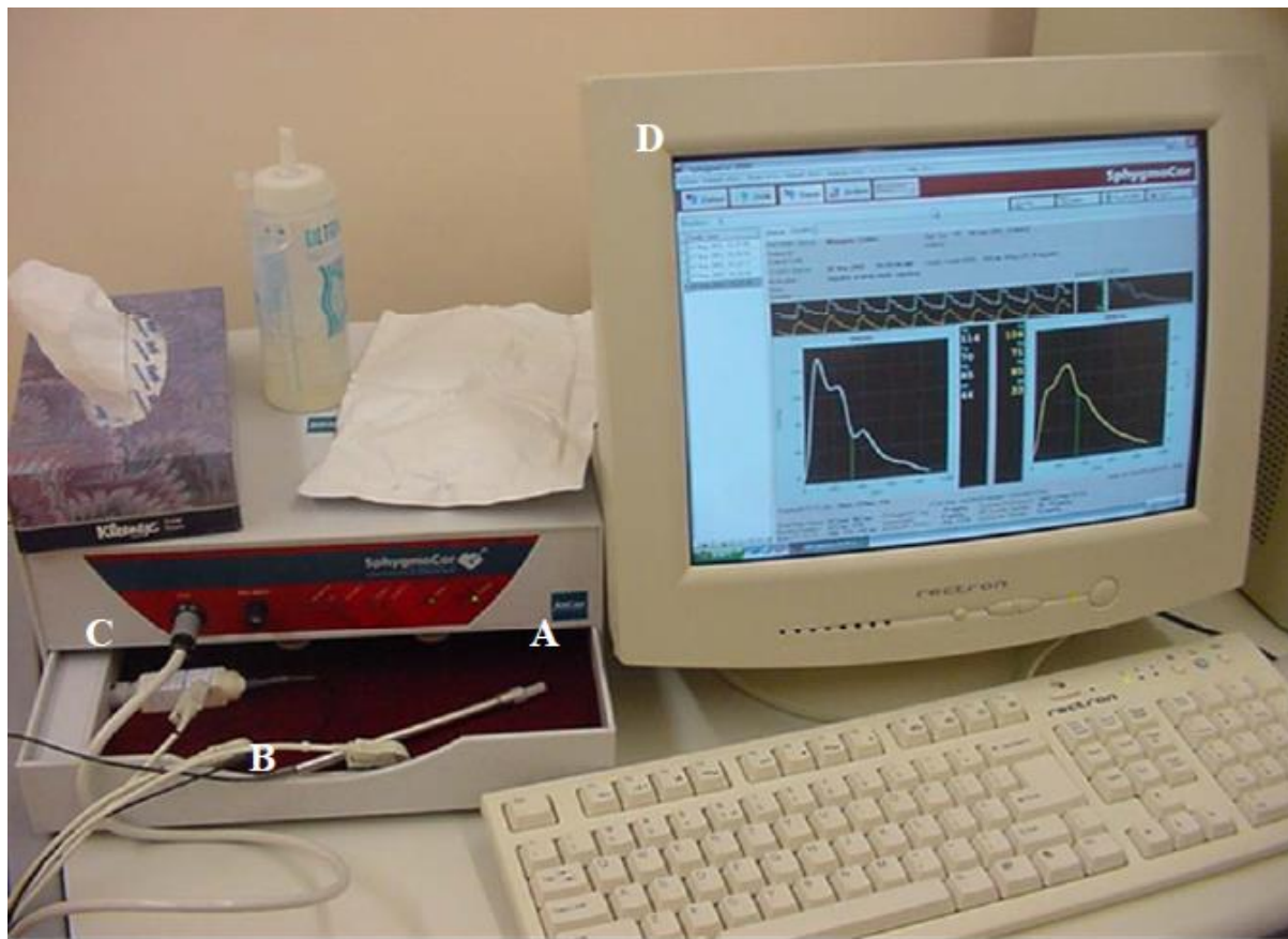
Figure 4.1: SphygmoCor device coupled to an applanation tonometer used to determine central (aortic) haemodynamics and aortic PWV
