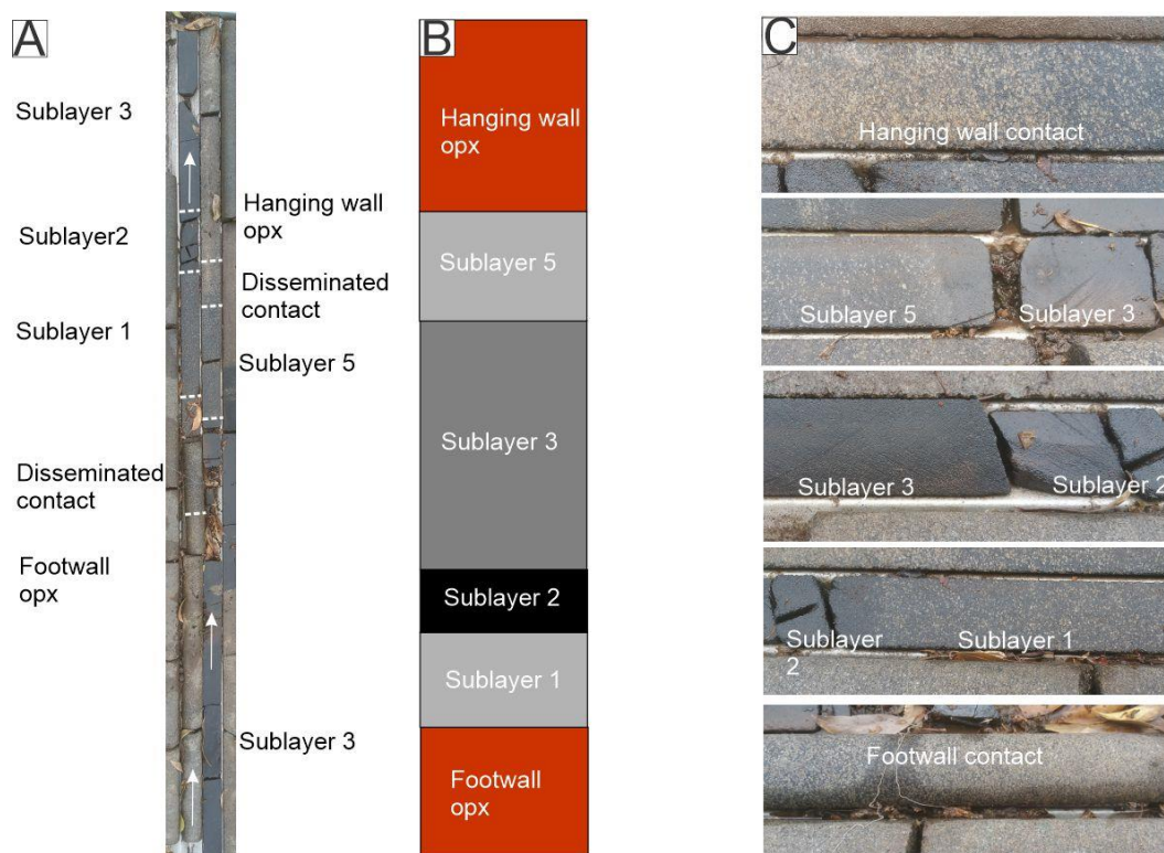
Figure 39: Overview of drill core WVS15, which was used for chemical analyses. (A) is a photograph of the LG6 chromitite as it appears in the drill core. The white arrows point upwards in stratigraphy and the white dotted lines show contacts. The abbreviation opx stands for orthopyroxenite in this figure. (B) is a stratigraphic column of the sublayers in the LG6 chromitite layer. (C) shows a detailed view of the contacts between the LG6 chromitite and its host rock orthopyroxenite, as well as between sublayers in the LG6 chromitite.
