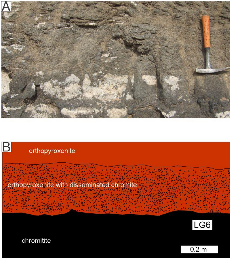
Figure 7: Photograph (A) and sketch (B) of disseminated chromite in the immediate hanging wall of the LG6 chromitite at Jagdlust. This structure is present in some outcrops of this location and differs from a gradational contact, as the area of orthopyroxenite with disseminated chromite exhibits sharp contacts to both the chromitite and the orthopyroxenite. The hammer in the photograph is 0.3 m long.
