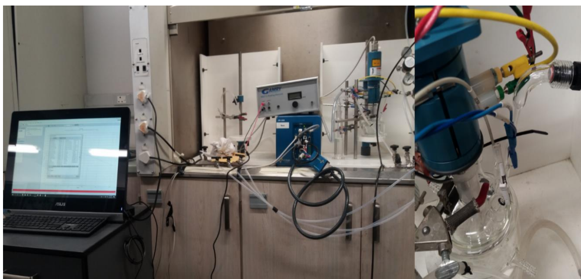
Figure 2.6: Three electrode setup showing RDE box, potentiostat, electrochemical cell and electrodes.
