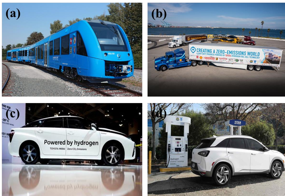
Figure 1.4: (a) PEMFC run passenger train from Germany, (b) Toyota PEMFC heavy duty truck, (c) Toyota Mirai fuel cell passenger sedan and (d) Hyundai Nexo crossover SUV running a hydrogen fuel cell. 38,45–47
