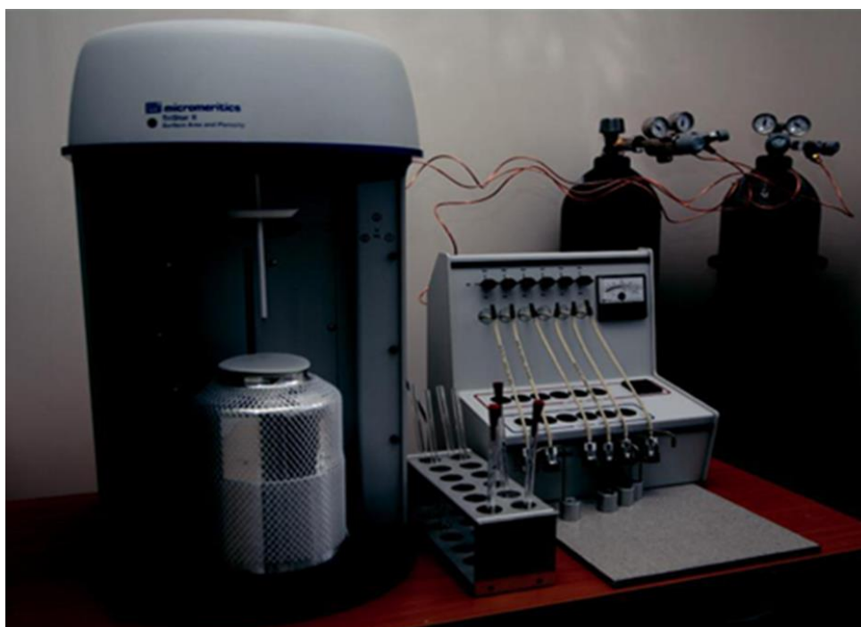
Figure 2. 10: A Tristar 3000 physisorption instrument.
