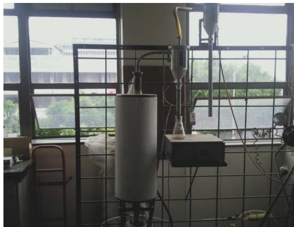
Figure 3.1 Vertical CCVD reactor set up used for the synthesis of MWCNTs
