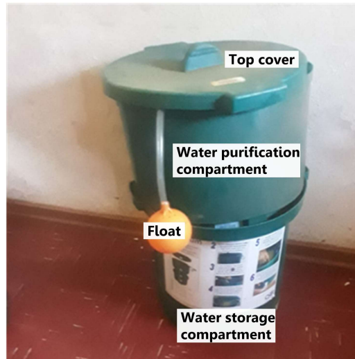
Figure 8: AmaDrum technological innovation at the Thambonkulu tribal authority hall showing the various components (Source: Author)
