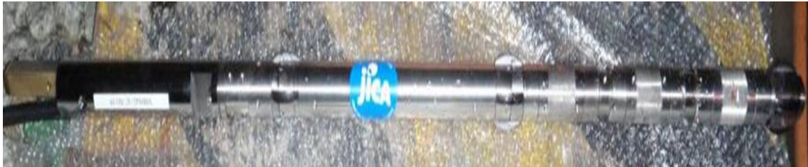
Figure 4: 5 Ishii 3-component strain-meter (Ogasawara, 2011)
