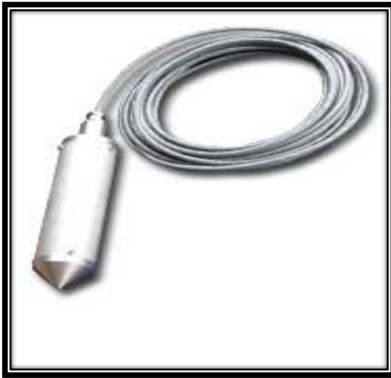
Figure 4: 6 Triaxial mine piezoelectric accelerometer (photograph courtesy of South Deep gold mine)
