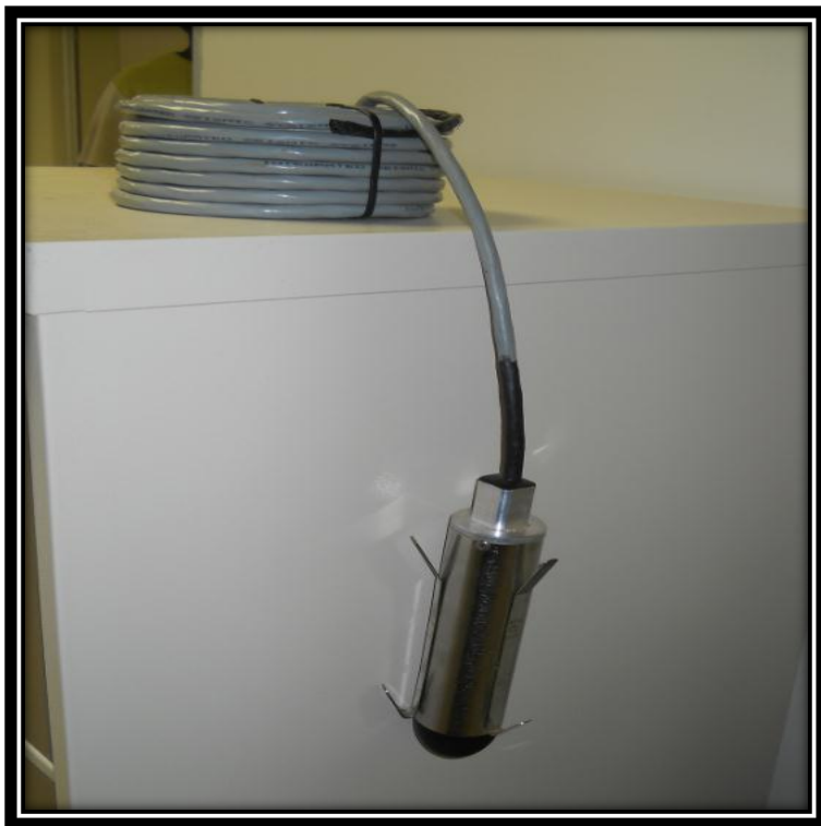
Figure 4: 7 4.5Hz Borehole geophone (photograph courtesy of South Deep gold mine)
