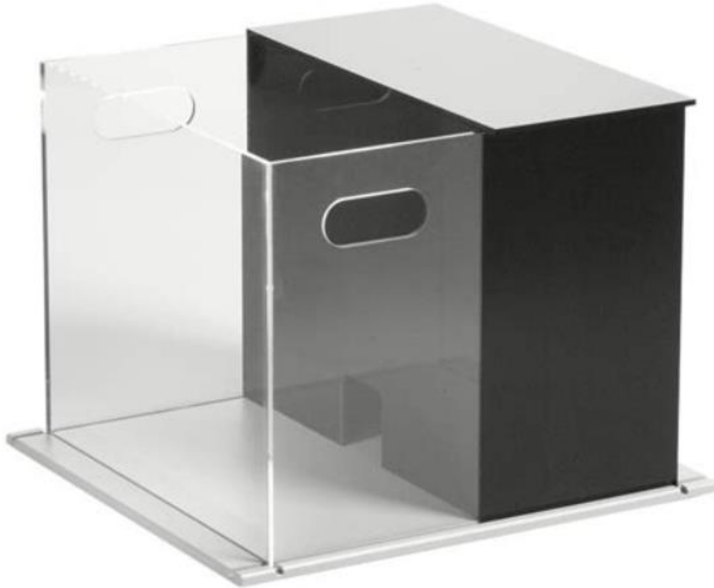
Figure 3.5: Schematic representation of the light dark box (Adapted from: https://brainstuff.org/blog/what-does-the-light-dark-box-test-measure )
