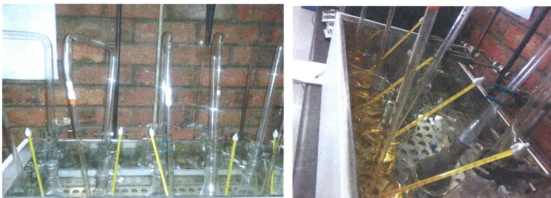
Figure(s) 21: Static Isothermal Method (spontaneous combustion liability test)
