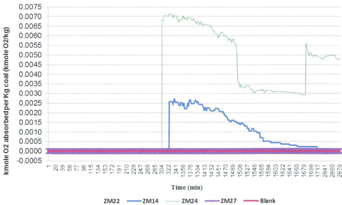
Figure 183: Smith-Glasser Oxygen absorption (ZM22, ZM14, ZM24, ZM27)
