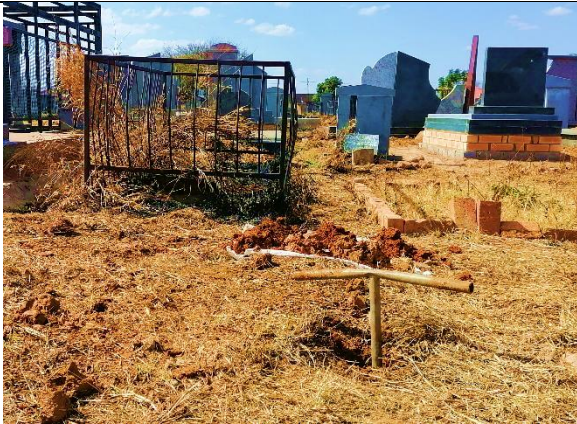
Photo 5: Hand auger drilling of MW3
