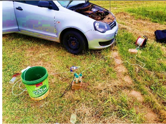
Photo 12: Connection between Abstraction well and flowthrough chamber
