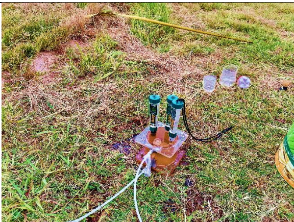
Photo 13: View of flowthrough chamber and water quality parameters
