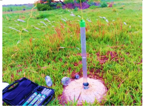
Photo 16: Groundwater sampling by bailing method in MW2
