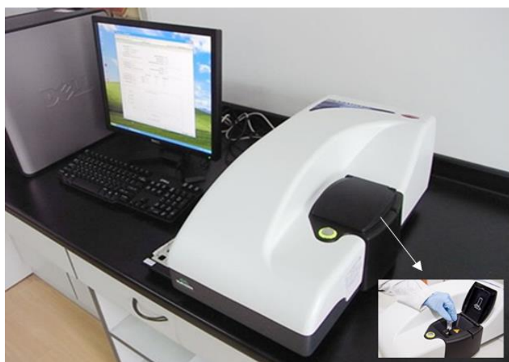
Figure 3. 10: Photograph of Zeta potential analyzer (Zeta sizer Nano series model) used.
