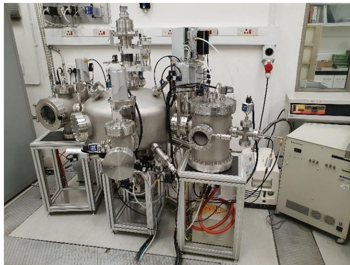
Figure 2. 16: Deposition vacuum chamber as set setup at the Nano-scale transport laboratory. School of Physics, Wits University.
