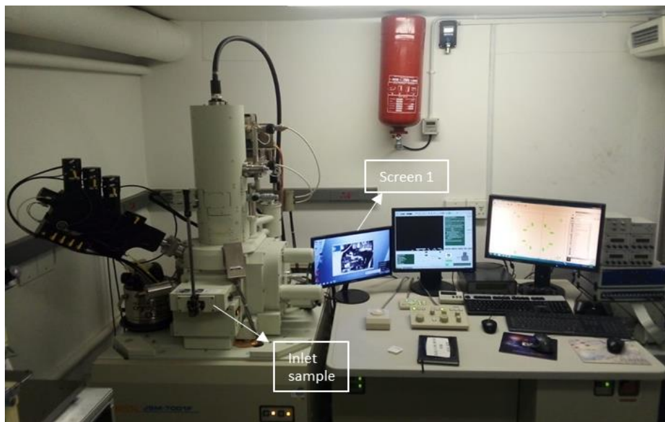
Figure 3. 6: SEM machine connected with electron beam lithography at the NSTP Laboratory, Wits University.
