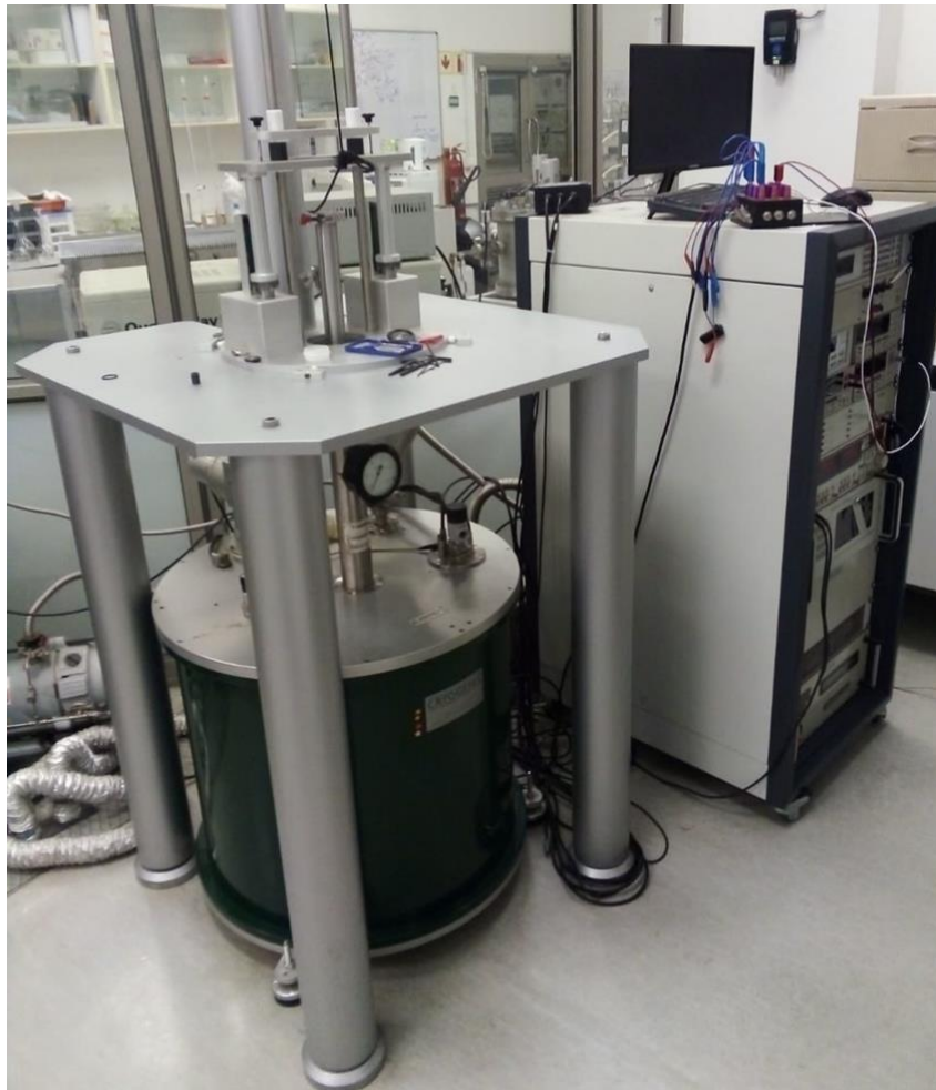
Figure 3. 13: Image of the Cryogenic high field system at NSTP laboratory, School of Physics, Wits University.
