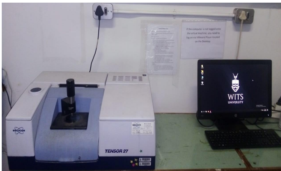
Figure 3. 9: Bruker Tensor 27 FT-IR spectrometer used in this project.
