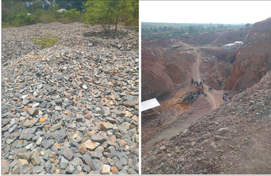
Figure 14: Poor rock stockpiling and massive land disturbance.
