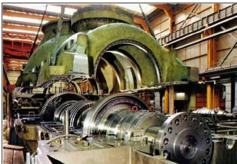
Figure 19 - Workshop Assembly of the Huntorf Turbine (BBC, 1990)
