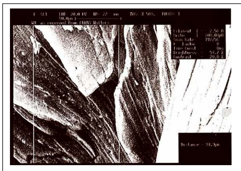
Figure 2-13 Scanning Electron Micrograph (SEM, magnification x 500) of graphene sheet clusters in highly ordered anisotropic petroleum coke (Clark, 1996)
