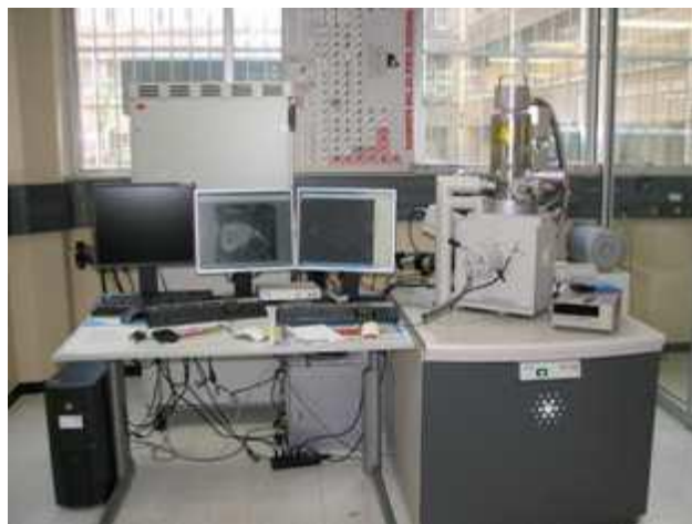
Figure 3-8: JEOL 7500F scanning electron microscope used to study the samples.
