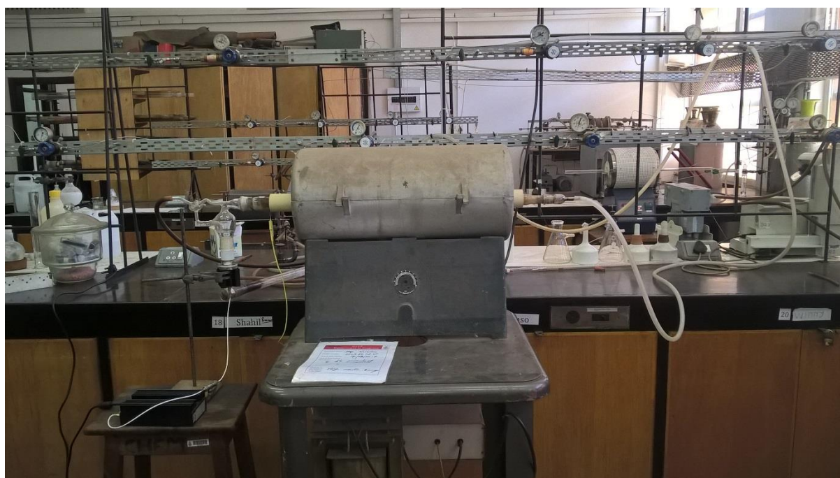
Figure 3-3: Experimental setup for C-GaN synthesis.
