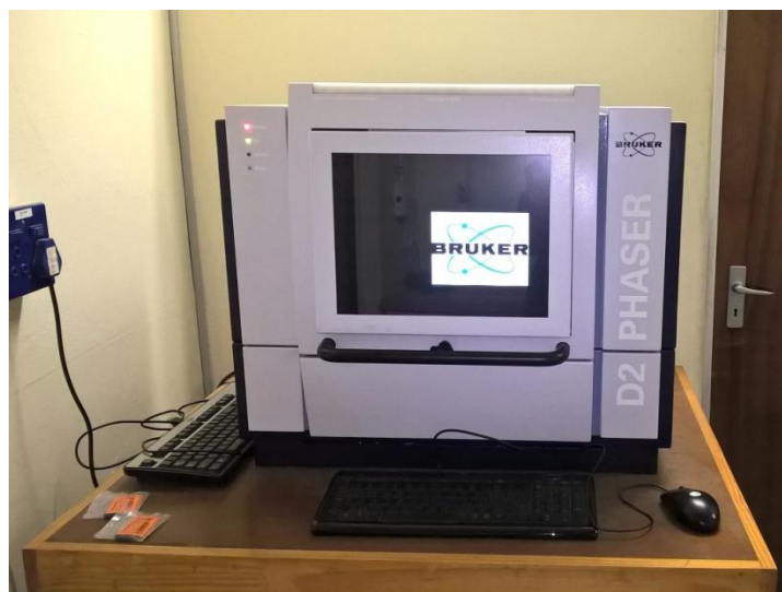
Figure 3-5: Bruker D2 Advance diffractometer.
