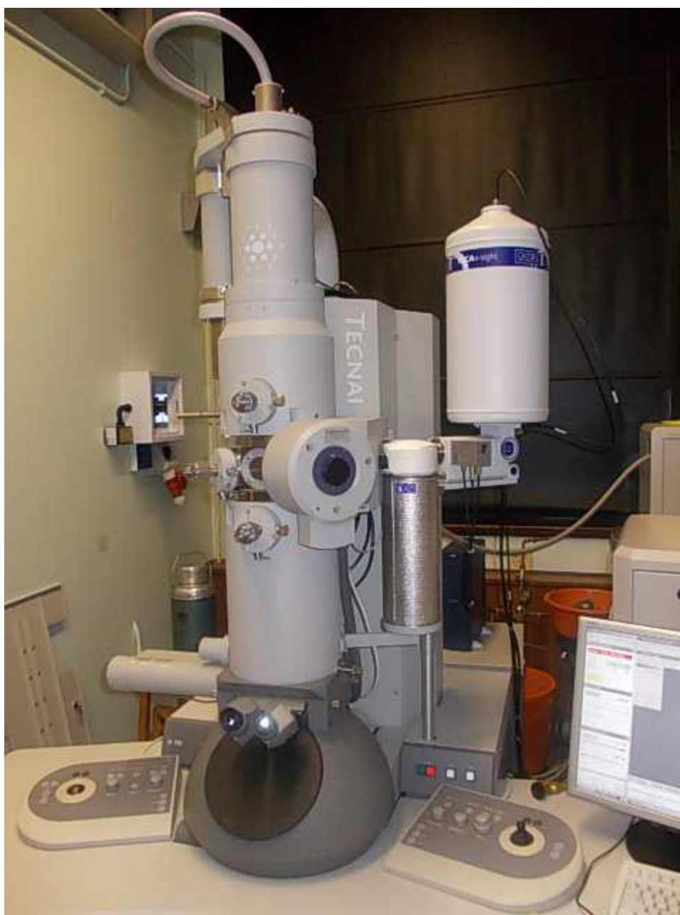
Figure 3-7: FEI Tecnai G2 Spirit electron microscope.
