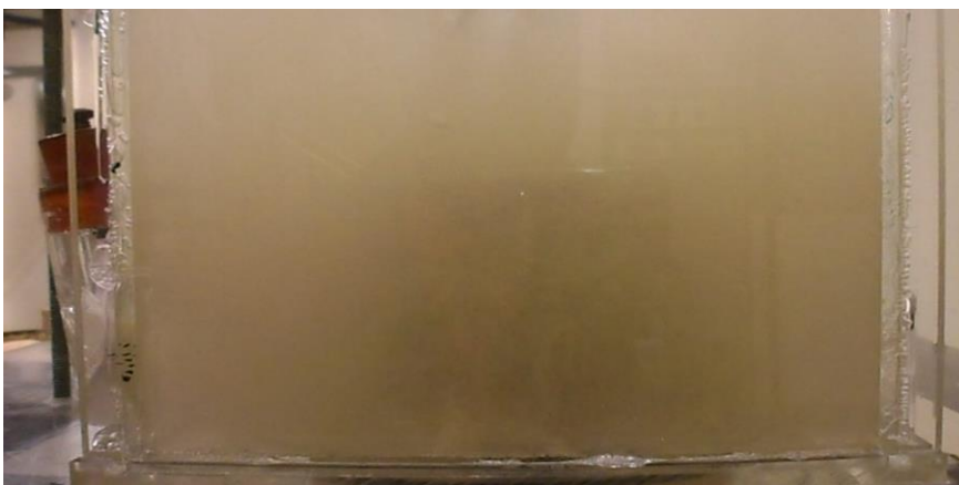
Figure 3.10c: Picture showing almost all sand particles suspended in the water agitator speed at 1500 rpm.
