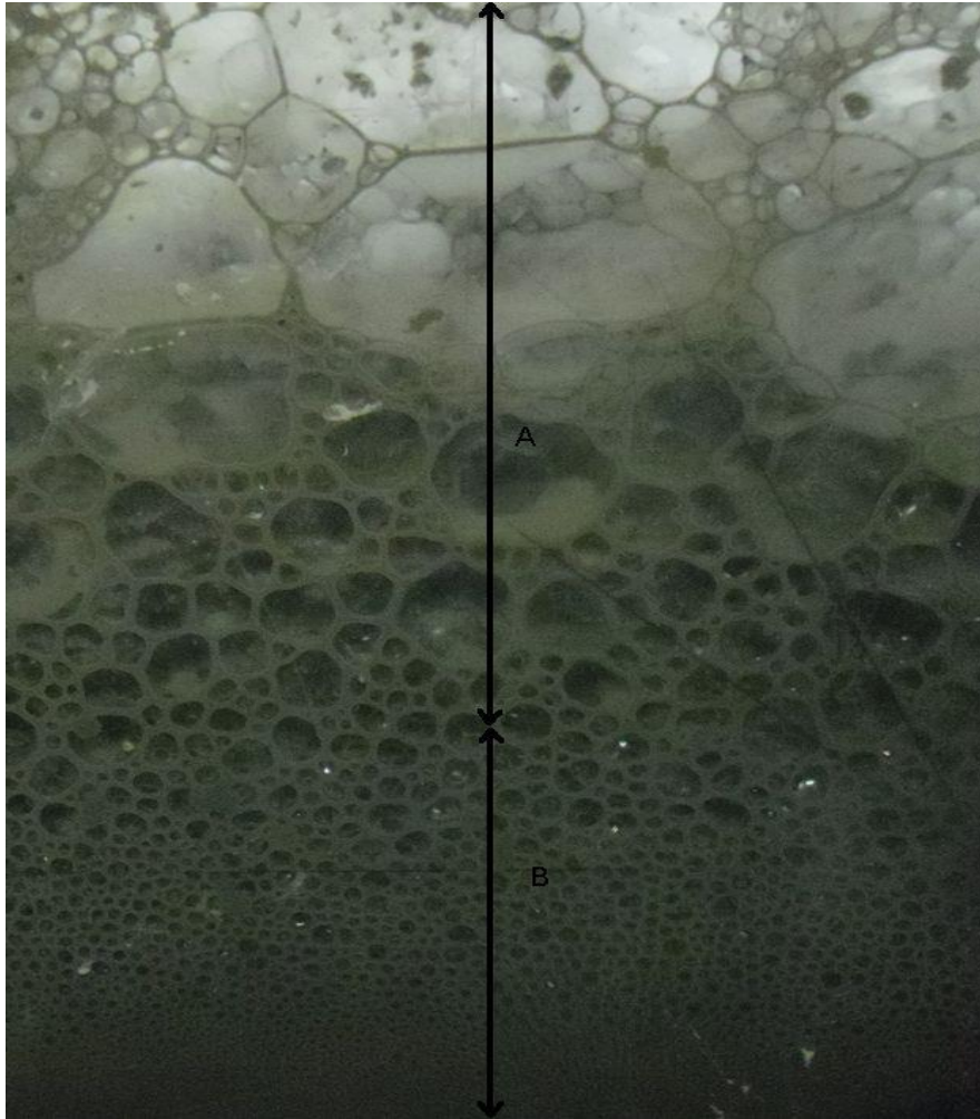
Figure 5.4: Picture showing variation in bubble sizes above the pulp-froth interface.
