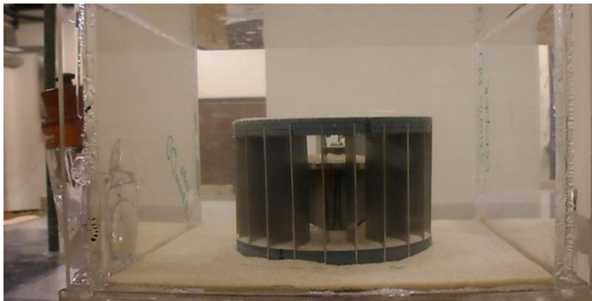
Figure 3.10a: Picture showing settled silica sand when the agitator is stationary
