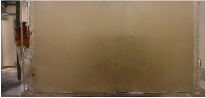
Figure 3.10c: Picture showing almost all sand particles suspended in the water agitator speed at 1500 rpm.
