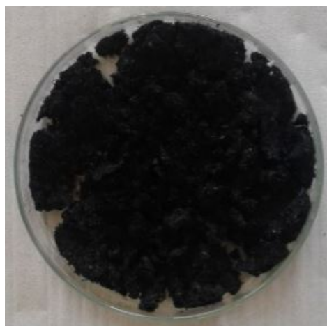
FIGURE 3.15: Dry functionalized SWCNTs.
