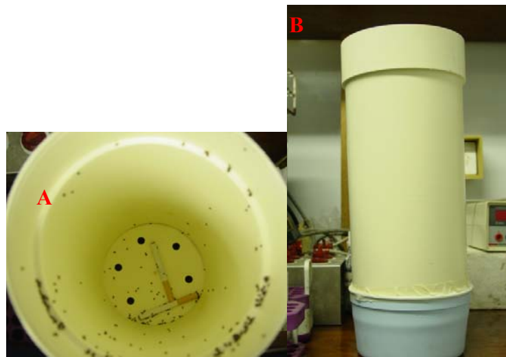
Figure 5.1 – Innovative sampling device designed to attract adult pests into collection area. A - shows a view from above of the MNS Tower where cigarettes were added as an attractant for fit tobacco beetles. B - illustrates assembled MNS Tower.
