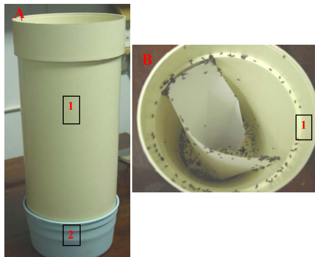
Figure 4.1 - Innovative Lure dubbed the MNS Tower– for selection of live adult insects from sieved population. A- Assembled tower with sieved insects in 2, the containment zone. B- View from the top showing wandering individuals gathering in 1, the collection chamber.
