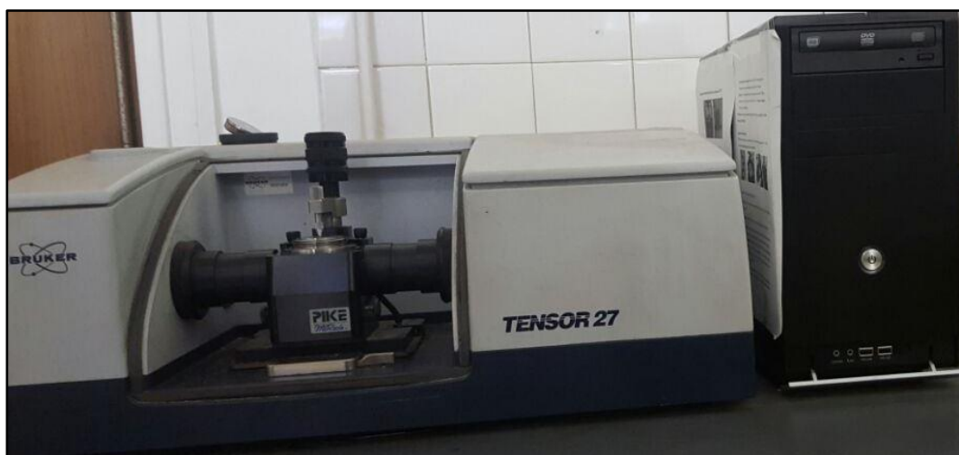
Figure 4. 16: Bruker TENSOR 27 FTIR Spectrometer.
