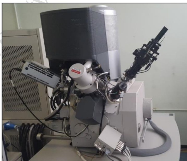
Figure 4. 4: FEI Nova Nanolab 600 FEG-SEM/FIB instrument.
