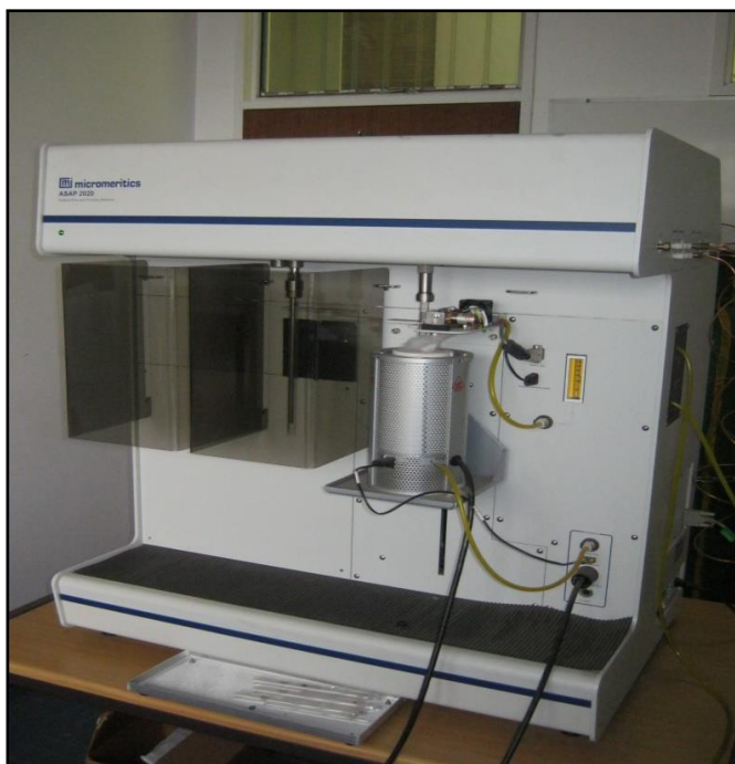
Figure 4. 10: Micromeritics ASAP 2020 chemisorption unit.
