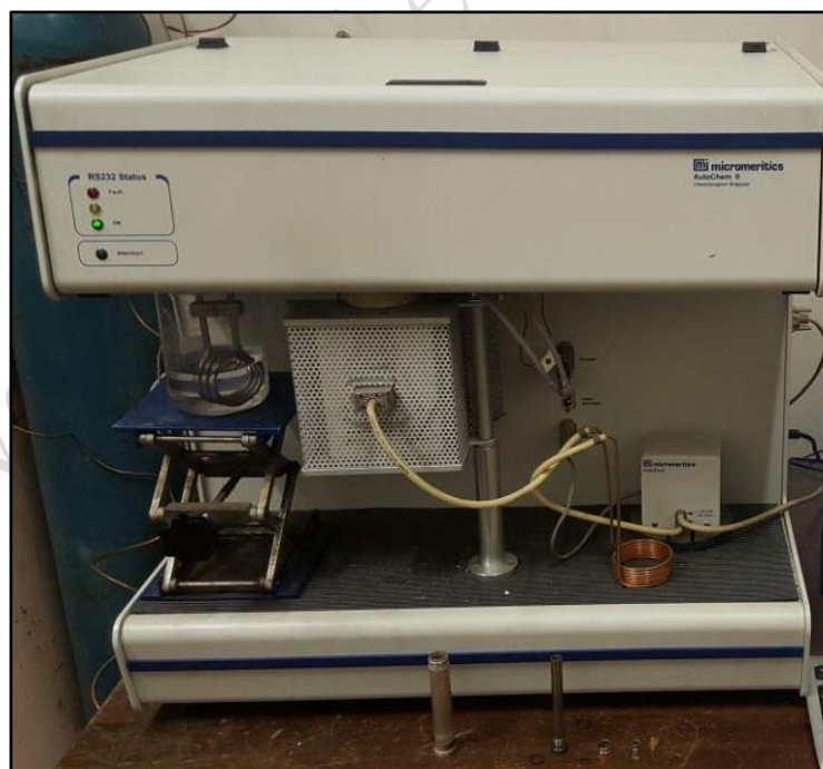
Figure 4. 12: Micromeritics AutoChem II instrument unit.
