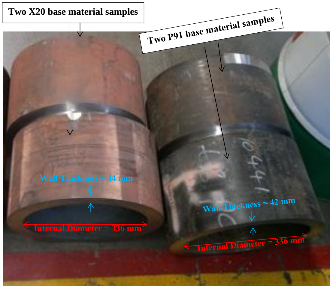
Figure 3.2: Photograph showing the X20 and P91 base materials pipe samples with their respective dimensions.
