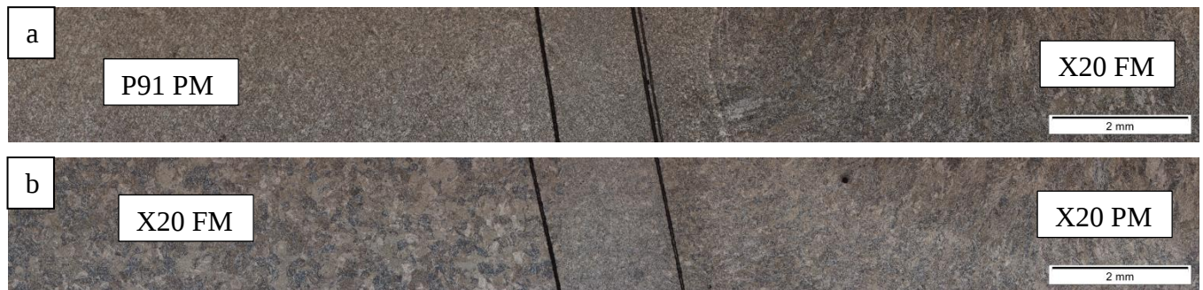
Figure 3.10: Stereo macrographs with scribe lines indicating where the HAZ samples were removed from the X20 weld filler material sample (a) P91 parent material side, (b) X20 parent material side.
