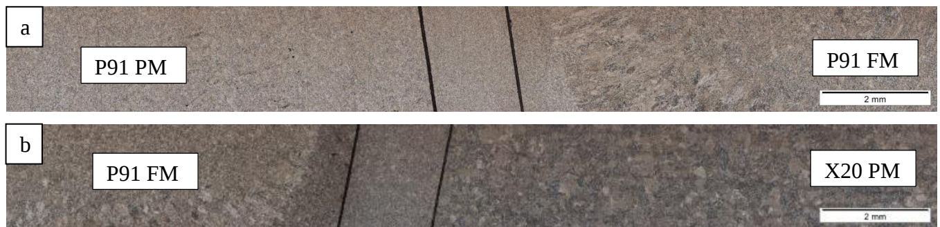
Figure 3.11: Stereo macrographs with scribe lines indicating where the HAZ samples were removed from the P91 weld filler material sample (a) P91 parent material side, (b) X20 parent material side.
